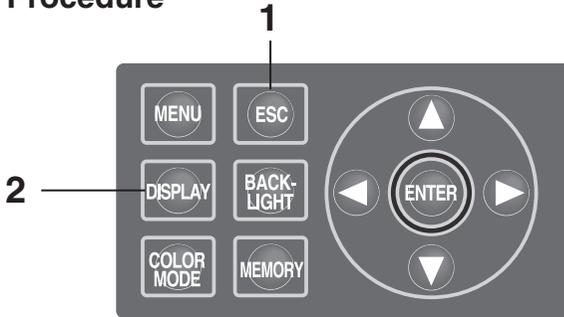
1. When the MENU or MEMORY screen is displayed, press **ESC** key to switch to the MEAS screen.
