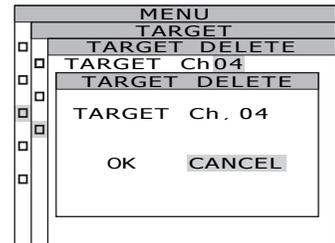
**5.-a-2.** To delete another target color continuously, repeat the steps 4 through 5-a-1. as necessary.
