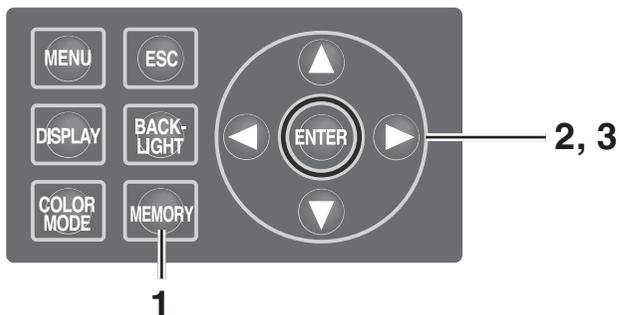
1. When the MEAS screen is displayed, press **MEMORY** key to switch to the **MEMORY** screen.
