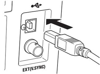
Communication interface in this instrument conforms to USB1.1.
