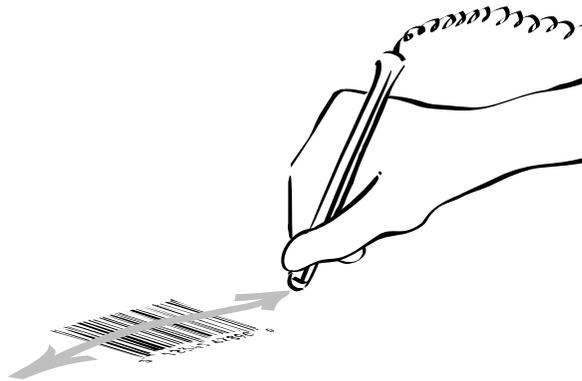
FIGURE 4. Scanning With the Wand
