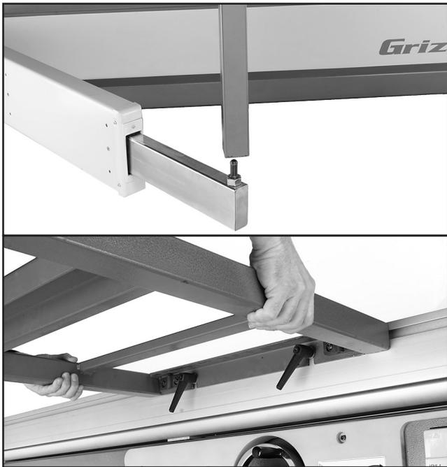
**Figure 42.** Installing the crosscut table.
