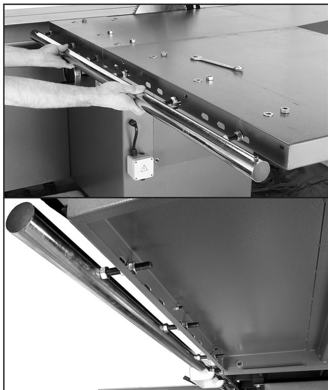
**Figure 22.** Installing the round rail.
