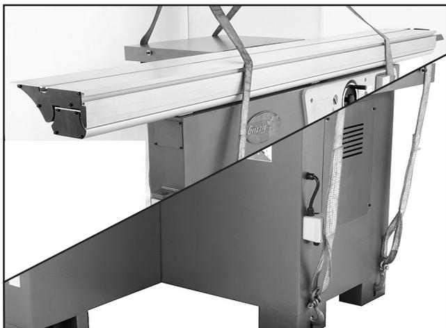
**Figure 9.** Lifting the saw base unit.
