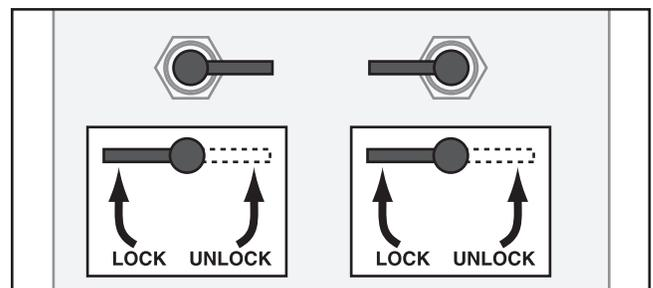
**Figure 4.** Configuration to extend the table beyond the regular stopping position.
