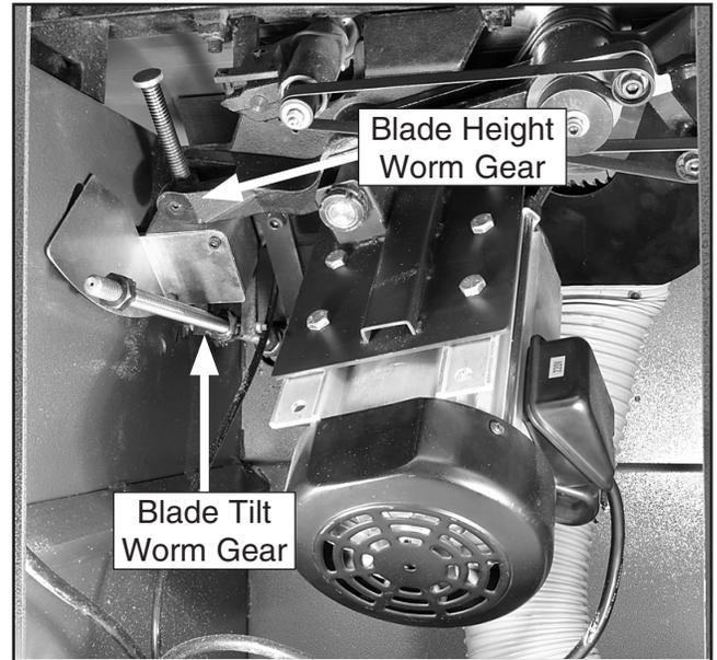
**Figure 79.** Gear lubrication.
