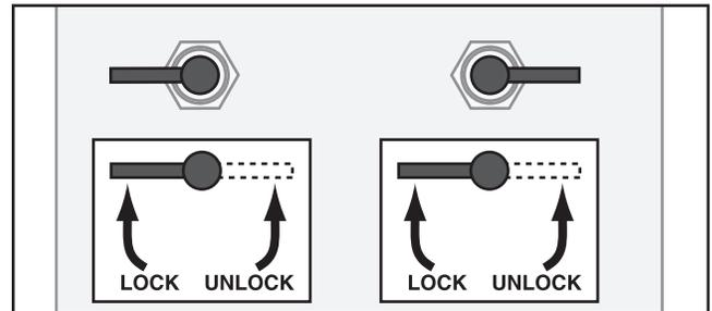
**Figure 2.** Configuration to lock the table so it is centered with the saw cabinet.
