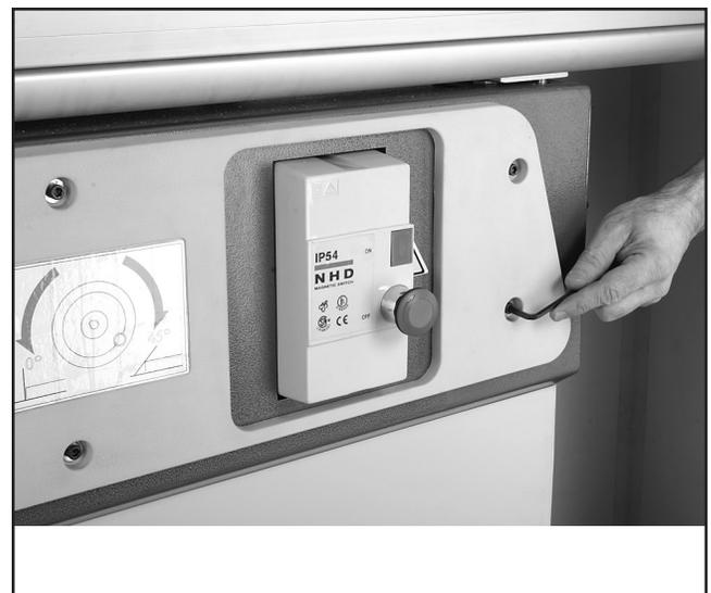
**Figure 6.** Control panel cover plate.
