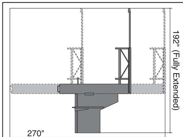
**Figure 10.** Working clearances.
