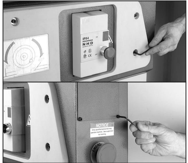
**Figure 17.** Removing cover plates.
