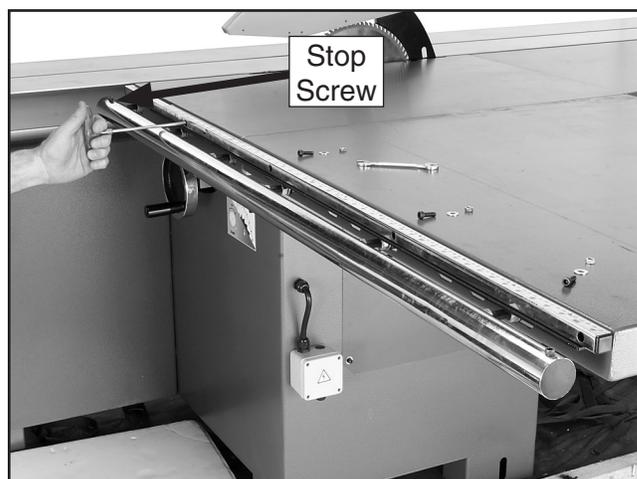
**Figure 23.** Attaching the scale.
