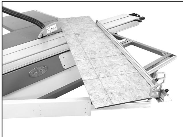
**Figure 64.** Example of miter cutting operation.
