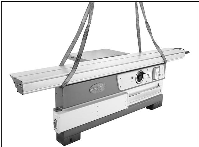
**Figure 16.** Installing the sliding table.
