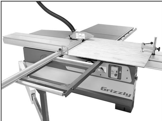
**Figure 50.** Rip cutting with the sliding table.
