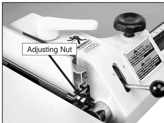
**Figure 24.** Aligning the round rail.
