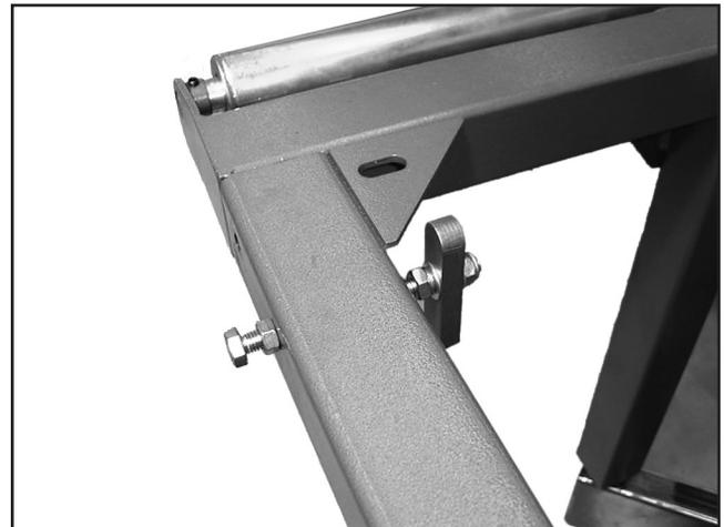
**Figure 44.** Crosscut fence adjustment screw.
