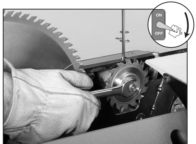
**Figure 34.** Installing the scoring blade.
