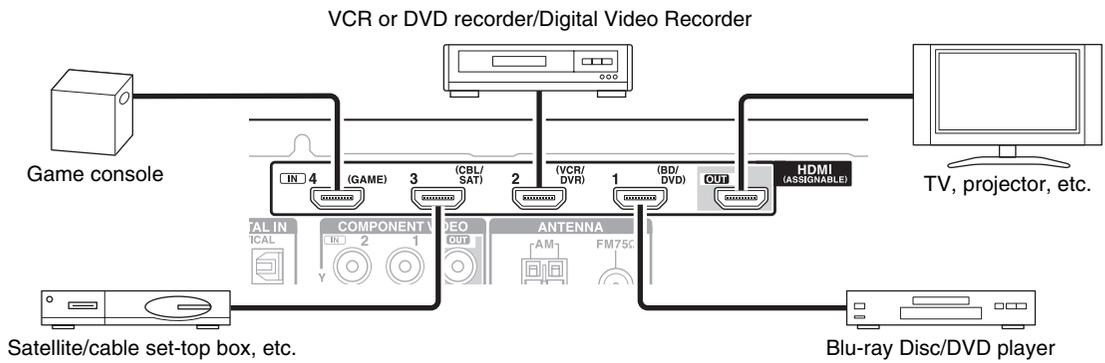
Connect your components to the appropriate jacks. The default input assignments are shown below.
