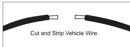
2. Twist one end of the vehicle's wire with the security module's wire.
