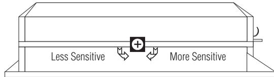
There is a Doubleguard® shock sensor inside the control unit. Adjustments are made via the rotary control as indicated above. Since the shock sensor does not work well when mounted firmly to metal, we recommend against screwing down the control module. The full trigger of the on-board shock sensor reports zone 2. (See *Table of Zones* section of this guide.)
