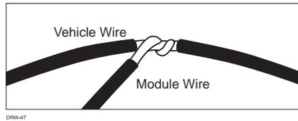
4. Completely insulate the connection with electrical tape.
