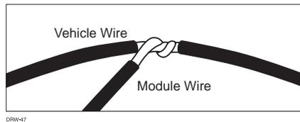
3. Solder the bare connection thoroughly using rosin core solder.
