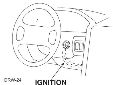
4. Turn the ignition key switch to the run position. If your meter reads (+)12V, go to the next step. If it doesn't, probe another wire.
