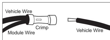
4. Insert the other end of the vehicle's wire into the other end of the butt connector and crimp securely.
