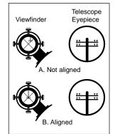
Fig. 13: Aligning the viewfinder. Note that objects appear upside-down and reversed left-for-right when observed in the viewfinder.
