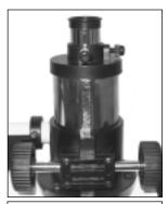
Fig. 14: Eyepiece and focuser assembly.
