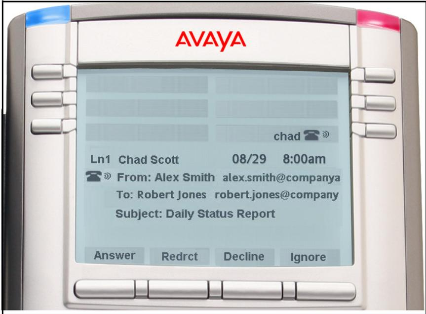
When the address or subject line is long, you can scroll by using the left and right navigation keys.
