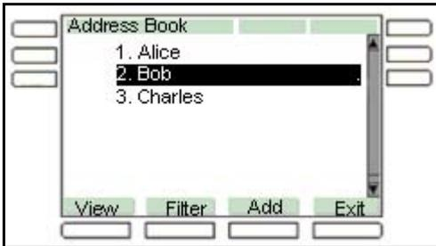
To view information about a contact use the navigation button to highlight a name, and then press the **View** context-sensitive soft key. The name, SIP address, and designation of contact or not as **Friend** appears. See [Figure 25 on page 163](#).
