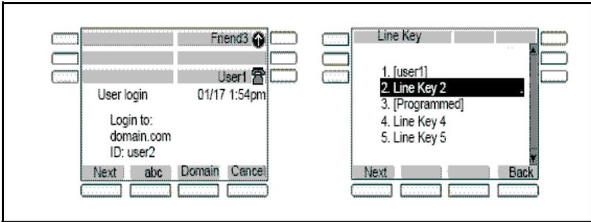
You can specify the Line Key to which the new account is associated. By default, the first unused key is selected. If the configured limit is reached on concurrent logins, then the selected login command displays an error message. The initial login message **login in process** displays during the login operation.
