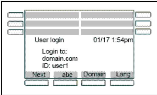
After you are logged in, the IP Deskphone displays the Idle screen. You can configure up to five profiles. If the limit is exceeded, then the least recently used profile is automatically deleted.
