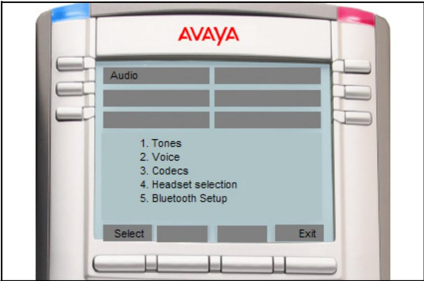
On the IP Deskphone, after you select the **Prefs**, **Audio**, and **Headset Selection** menu items, use the headset screen to select the desired headset and corresponding functional parameters. [Figure 21 on page 108](#) displays the headset screen.
