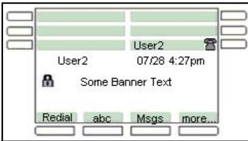
[Figure 8 on page 70](#) is an example of a secure connection when you are on an active call. The security icon is visible on the IP Deskphone screen.
