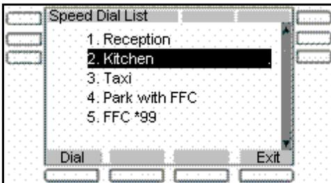
The Speed Dial List screen displays all the speed dial list entries provisioned. The displayed list items are based on the provisioned list as well as the current Idle/Mid-call state of the IP Deskphone. After you invoke the speed dial list while the IP Deskphone is idle, only Speed Dial List entries that are configured to IDLE are displayed. Similarly, only items marked as MID CALL are displayed if the Speed Dial List is invoked while the IP Deskphone is in a call.
