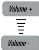
Use the **Volume control** buttons to adjust the volume of the ringer, handset, headset, speaker, and the Handsfree feature. Press the top button to increase the volume, and press the bottom button to decrease the volume.
