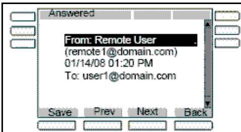
Call logs and IM logs provide many ways of initiating a call to the address identified by the selected entry, such as lifting the handset. In most cases, the primary account is used. However, if you press a line key to initiate the call, the call uses the account associated with the line key.
