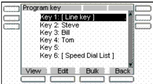
A feature key provisioned for use as a Speed Dial List has a similar appearance to all other programmed feature keys on the idle screen (or in-call screen). The label used for the selected key is provided through provisioning.
