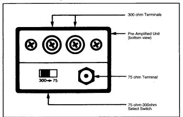
When coaxial cable is used it is terminated with an "F" connector and connected to the 75 ohm terminal on the pre-amplifier and the 75 ohm terminal on the amplifier unit labeled "to amplifier".
