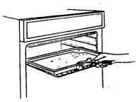
Adjust the grid and grill pan runner position to allow for different thicknesses of food. Position the food closer to the element for faster cooking and further away for more gentle cooking.
