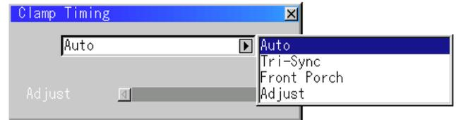
According to the signal, this function sets the detection position (i.e., clamp position) of the black level reproduction of the analog input signal. Normally this is not used.
