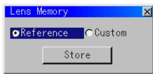
The Lens Memory function stores the adjusted values when using shift, focus\* and zoom buttons on the projector cabinet or the remote control for a specific signal.
