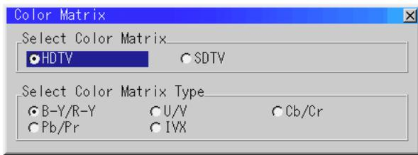
First, select an appropriate color matrix for your input signal, either HDTV or SDTV. Then select an appropriate matrix type from B-Y/R-Y, U/V, Cb/Cr, Pb/Pr or IVX.
