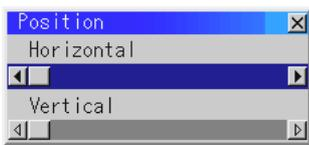
Adjusts the image location from left to right. This adjustment is made automatically when the Auto Adjust is turned on.
