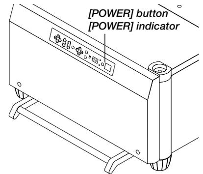
**NOTE:** Immediately after turning on the projector, screen flicker may occur. This is not a fault. Wait 3 to 5 minutes until the lamp lighting is stabilized.
