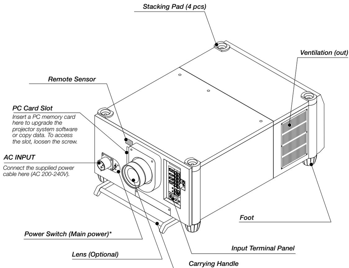
\* To turn on the main power to the projector, press the switch to the ON position (I) and the POWER indicator on the rear panel will turn orange in color. Press to the OFF position (0) to turn the main power off.
