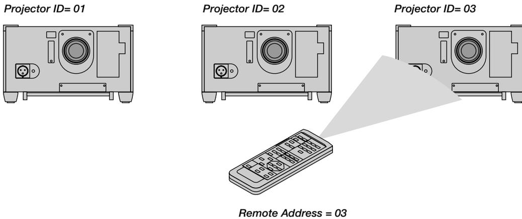
You can daisy-chain multiple projectors and operate them separately with the same remote control in wired operation.
