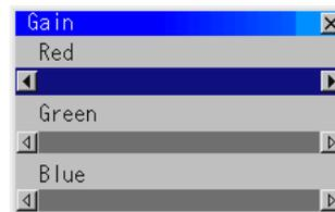
This feature adjusts the input level of the signal. This must be done to each color: R, G, and B.
