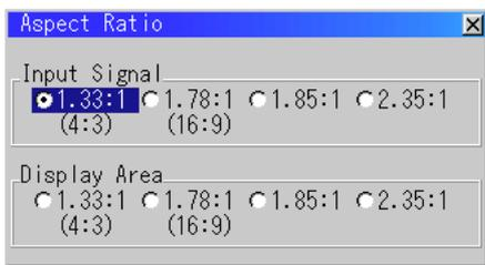
You can select the aspect ratio for input signal and display area respectively. Select the appropriate aspect ratio using the SELECT ◀, ▶, ▲, or ▼ button.
