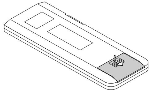
2. Align and insert the batteries according to the (+) and (-) indications inside the case.
