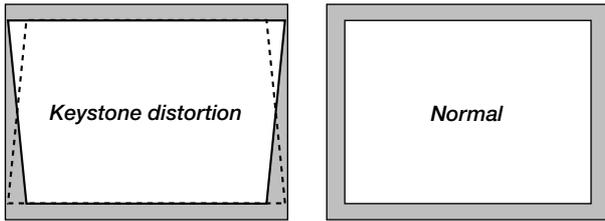
Keystone is the distortion of a projected image that usually creates a wider top than bottom. Aiming a projector upward on a wall rather than straight at a wall creates this distortion. Use the ◀ or ▶ buttons on the slide bar to correct this keystone (trapezoidal) distortion.
