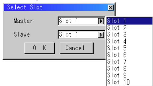
Use the SELECT ▲ or ▼ button to select the master slot number from 1 to 10 and then the slave slot number from 1 to 10 on the Select Slot menu. Select OK and press ENTER.
