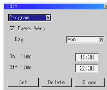
3. Set the Week, Day, On-Time and Off-Time using the Select buttons and Source buttons (1 thru 10). To cancel the on-time or off time, use Delete.
