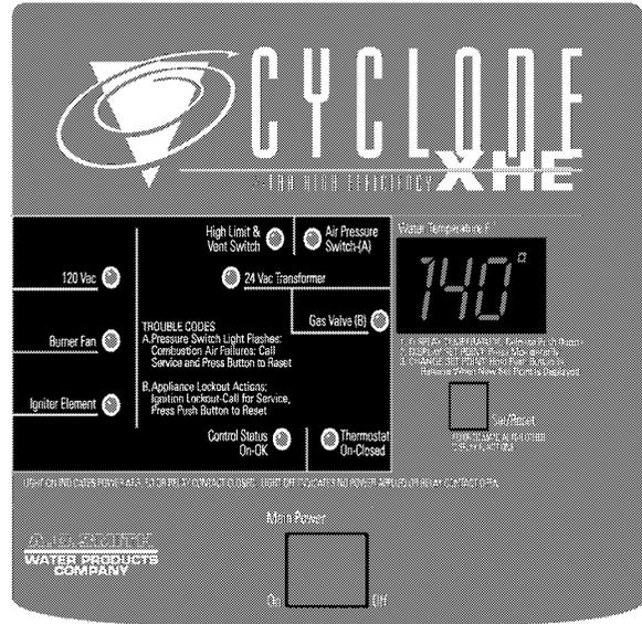
The water temperature inside the tank must be below the current temperature setting to activate a call for heat. Pressing the Set/Reset button approximately 4 – 6 seconds after powering up the water heater will reveal the current temperature setting. See the instructions below for how to view or change temperature settings.
