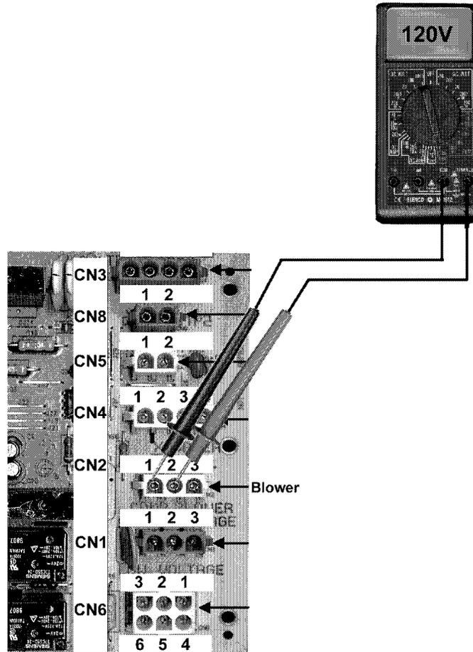
**STEP 8A:** CHECK FOR 120 VAC TO BLOWER FROM CN2 PLUG PIN 1 AND 2.
