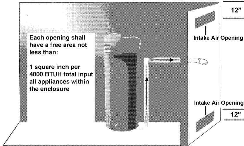
A fresh supply of make-up air for combustion can be supplied to the heater through make-up air openings, which directly communicate with the outdoors. Two openings are required — one within 12 inches of the top of the enclosure and one within 12 inches of the bottom of the enclosure. Each opening shall have a free area of not less than 1 square inch per 4000 BTUH of the total input of all appliances within the enclosure.
