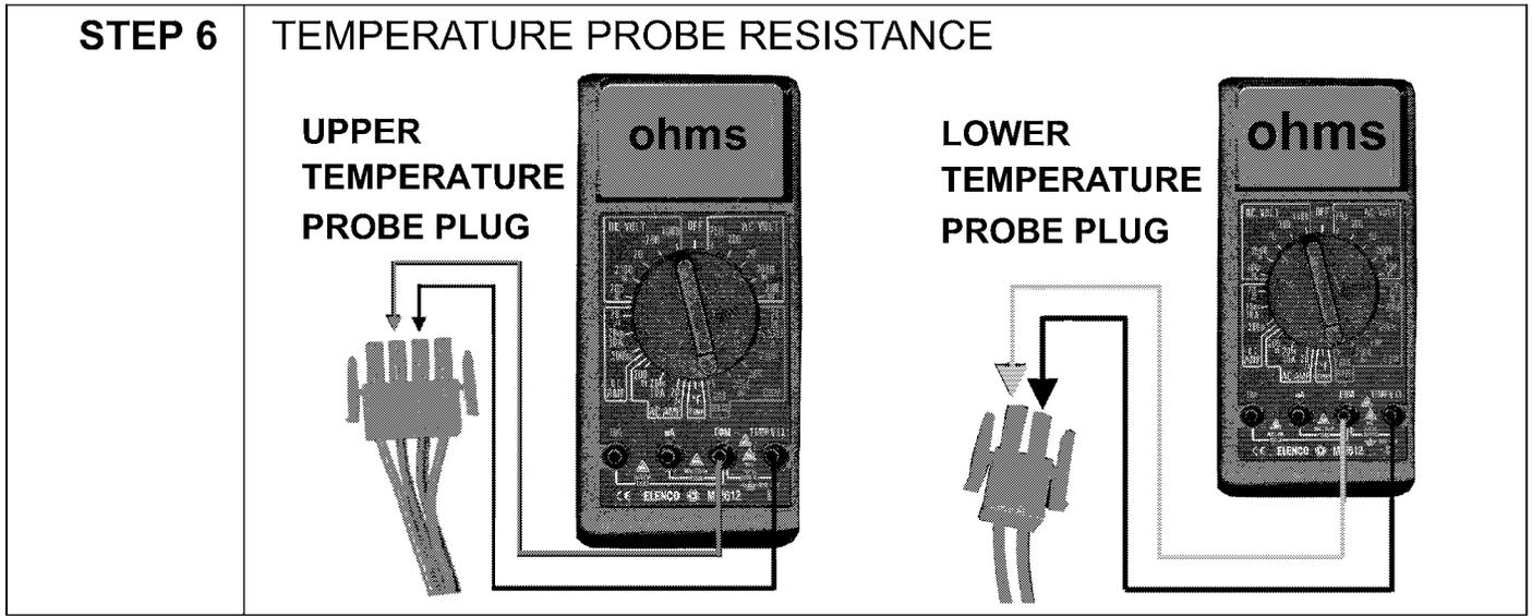
**STEP 6:** CHECK RESISTANCE OF THERMISTOR IN UPPER AND LOWER TEMPERATURE PROBES.
