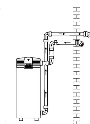
SEALED DIRECT VENT SIDEWALL
