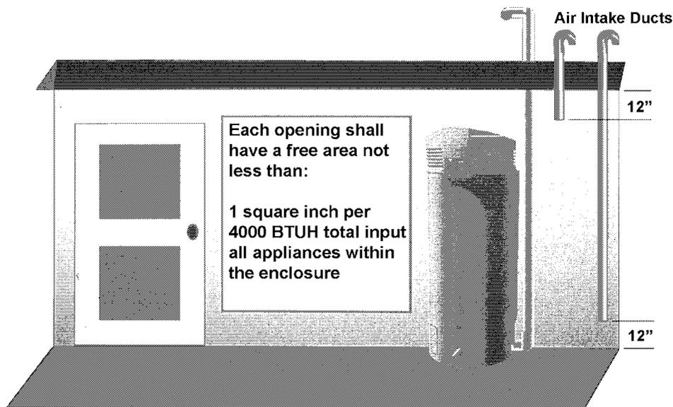
Often it is more practical to install vertical make-up air ducts to the outdoors. Again, two openings are required — within 12 inches (30 cm) of the top of the enclosure and one within 12 inches (30 cm) of the bottom of the enclosure. Each opening shall have a free area of not less than 1 square inch per 4000 BTUH of the total input of all appliances within the enclosure.
