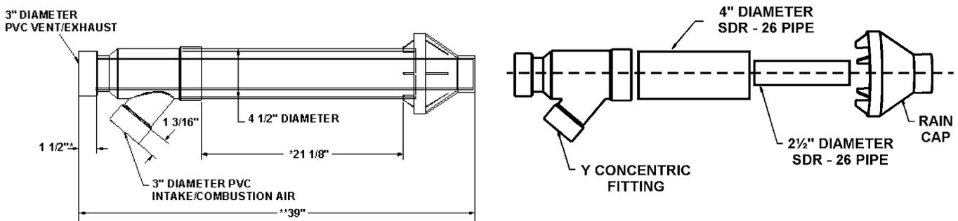
Dimension 21 1/8 in. may be lengthened to 60 in. maximum. Dimension 21 1/8 in. may also be shortened by cutting the pipes, provided in the kit, to 12 in. minimum. Dimension 39 will change accordingly as dimension 21 1/8 in. is lengthened or shortened
