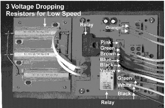
3 Voltage Dropping Resistors for Low Speed
