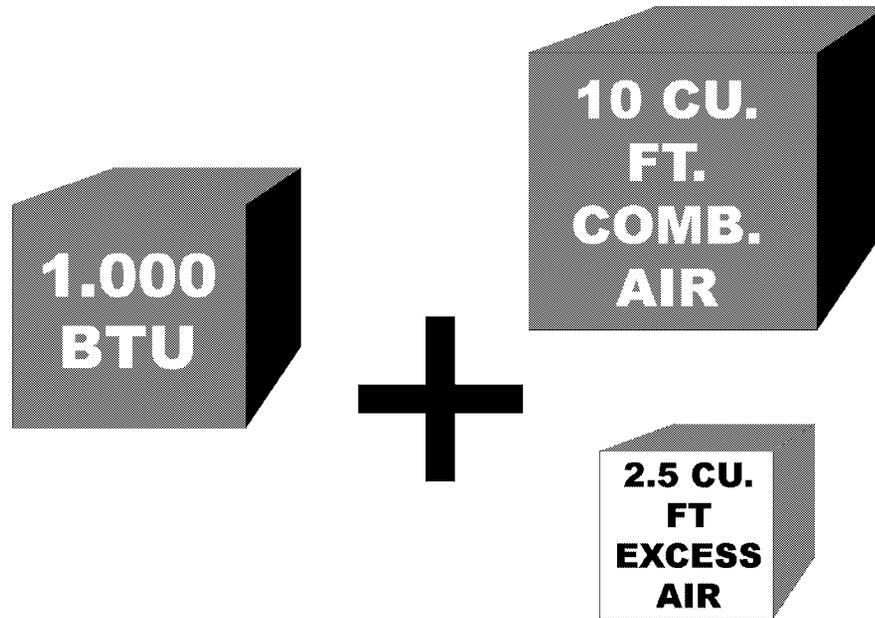
Stoichiometric or theoretical complete combustion requires 10 cubic feet of air per 1000 BTUH of gas input. The National Fuel Gas Code also recommends an additional 2.5 cu.ft. of “excess air”. This 12.5 cu.ft. minimum supply air per 1000 BTUH input applies to natural and propane gas models.
