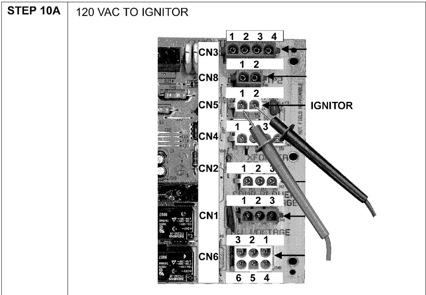
**STEP 10A:** CHECK FOR 120 VAC TO IGNITOR FROM PIN 1 AND 2 ON CONTROL BOARD TERMINAL CN5.
