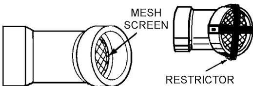
**WARNING** WHEN THE UNIT IS TO BE SETUP AS A DIRECT VENT, THE MESH SCREEN MUST BE REMOVED. THE INLET VENT PIPE MAY THEN BE GLUED TO THE AIR INTAKE (see following Figure) PROVIDED ON THE UNIT.
