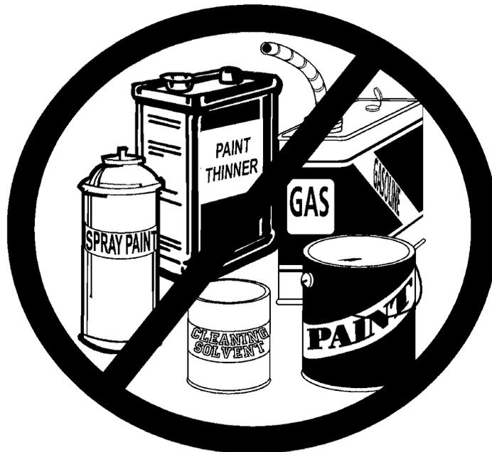
Flammable items or pressurized containers or any other potentially hazardous articles must never be placed on or adjacent to the heater. Open containers of flammable material should not be stored or used in the same room with the heater or in the area of the exterior air intake of a direct vent installation. Direct venting **does not** eliminate the need to remove flammable or corrosives from the area surrounding the heater.
