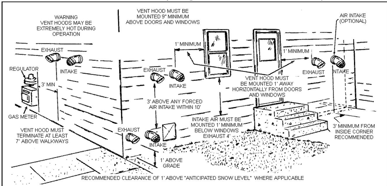
When multiple units are directly vented through a wall, all intake vent terminals must be no lower than the highest exhaust vent terminal.
