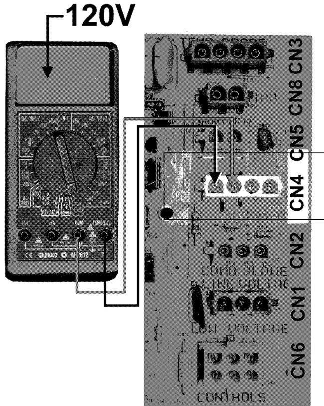
**STEP 2:** CHECK FOR 120 VAC TO TRANSFORMER FROM PIN 1 AND 2 ON CONTROL BOARD CN4 TERMINAL.
