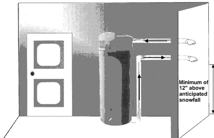
This model is approved for direct venting either horizontally or vertically or conventional venting horizontal or vertical. Direct venting avoids using room air for combustion and eliminates the need for additional air intake ducts.
