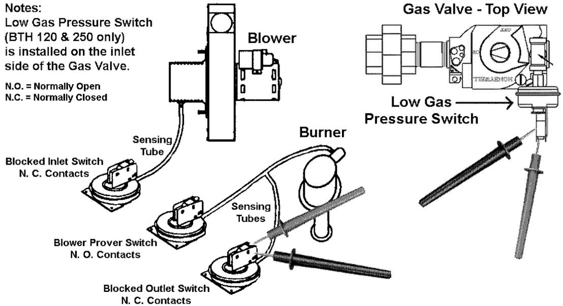
**STEP 7: CHECK FOR CONTINUITY BETWEEN PRESSURE SWITCH TERMINALS WITH WIRES REMOVED.**
