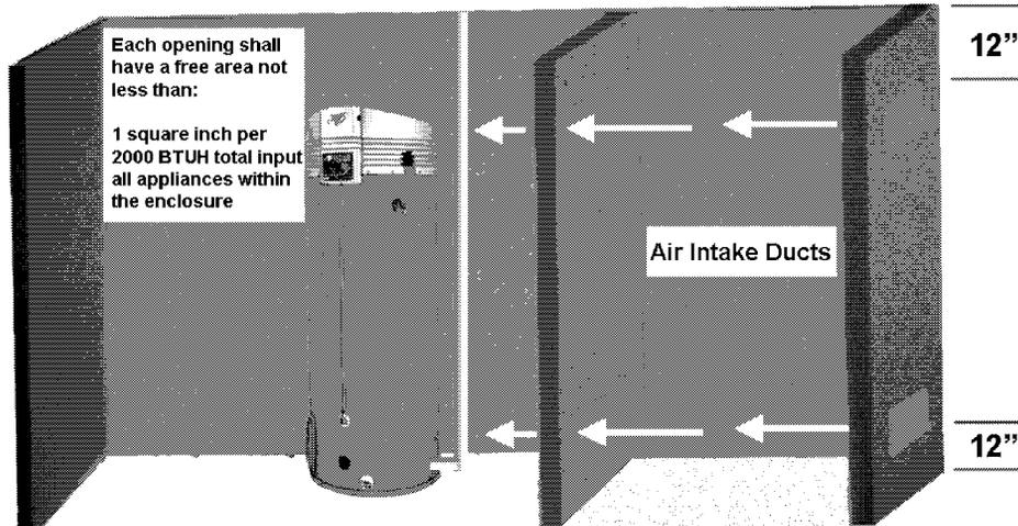
When the heater is installed in an interior room with no roof access for vertical ducts, horizontal make-up ducts should be installed. When using horizontal ducts, two openings are required - within 12 inches (30 cm) of the top of the enclosure and one within 12 inches (30 cm) of the bottom of the enclosure. Each opening shall have a free area of not less than 1 square inch per 2000 BTUH of the total input of all appliances within the enclosure.
