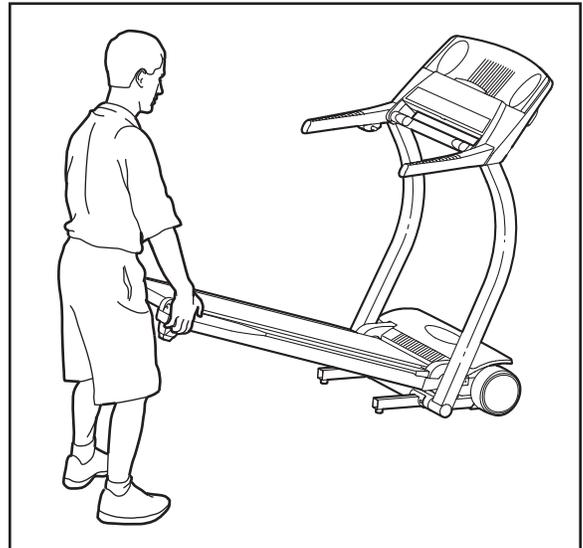
2. Move your right hand to the position shown and hold the treadmill firmly. Using your left hand, pull the latch knob to the left and hold it. Raise the treadmill until the foot rail is past the latch pin. Slowly release the latch knob. **Make sure that the foot rail is securely held by the latch pin.**
