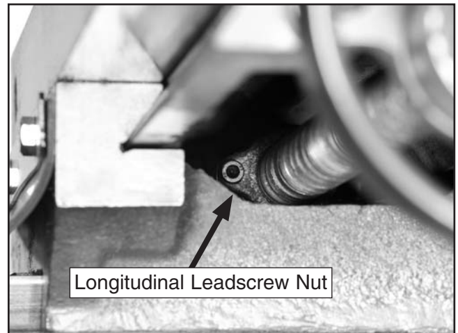
Figure 53. Longitudinal leadscrew nut (viewed from underneath the table on the left side).
