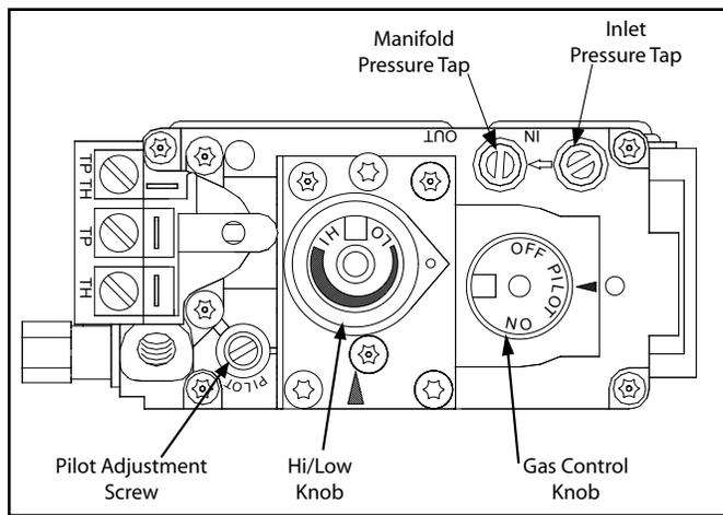
**Figure 37: Fully Labeled Gas Valve.**
