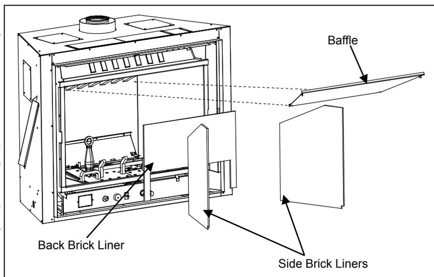
**Figure 38: Cast Iron Brick Liner Installation.**
