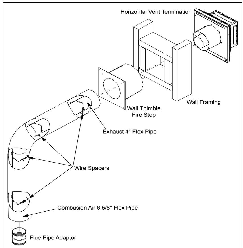
**Figure 22: Installation of Fireplace Horizontal Vent Kit.**
