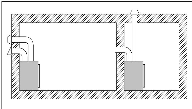
Figure 34. More Ducting Options; ducted to outside & to another room on an interior wall.
