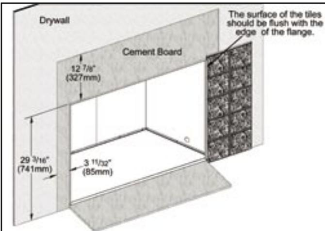
Figure 16. Dimensions Facing Around Opening.
