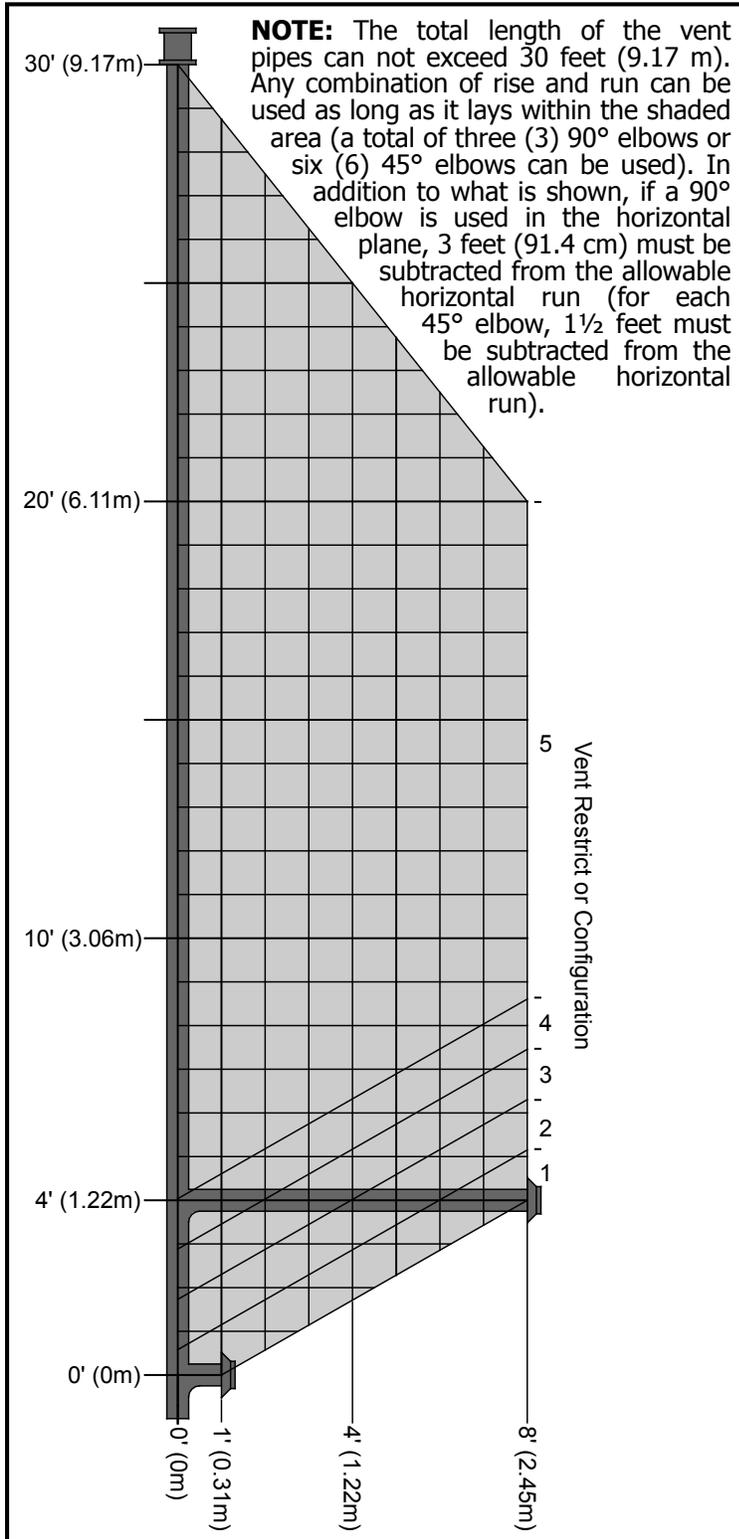
Figure 25. Possible Vent Configurations
