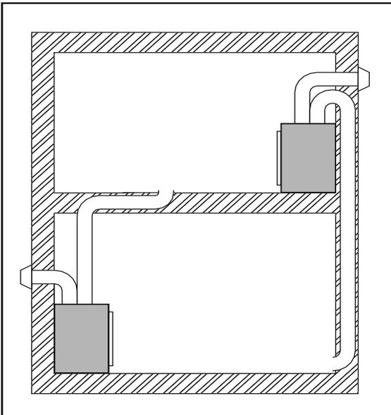
Figure 33. Ducting Options; ducted from upper floor to lower floor & from lower floor to upper floor.
