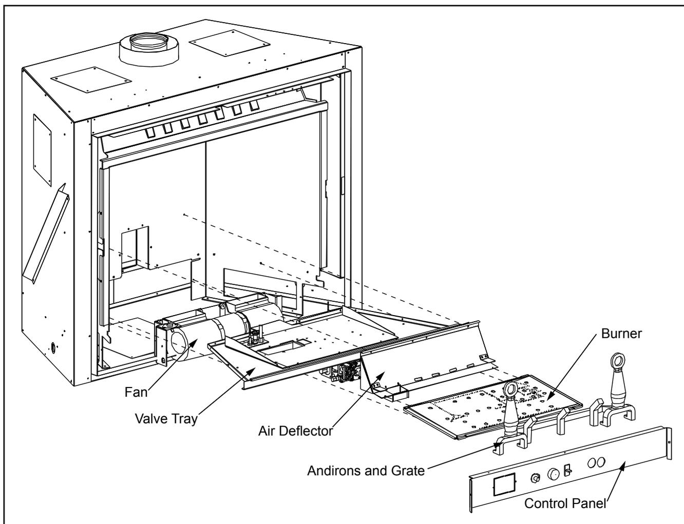
Figure 45: Removal of DV42DX Burner and Fan.
