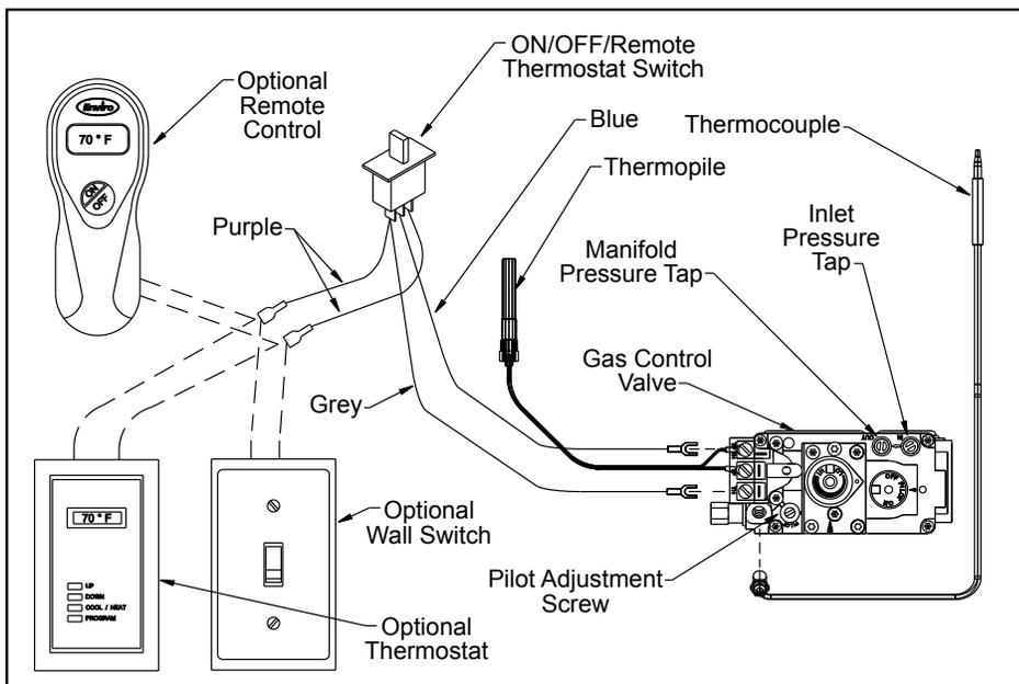
Figure 36. Wiring Diagram For Gas Valve.
