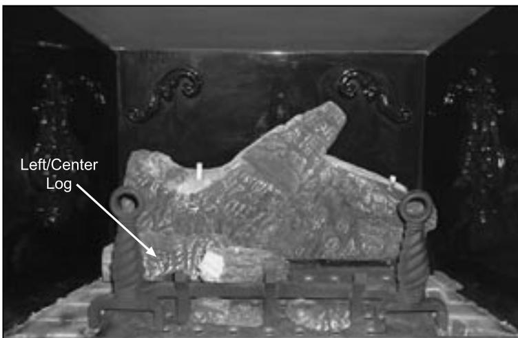
**Figure 40: Second Stage Log Set Installation.**
