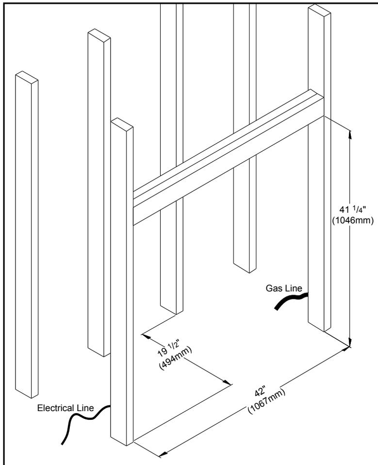
**Figure 10. Dimensions for Framing the Firebox.**
