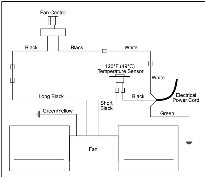
Figure 35. Wiring Diagram For Fan Control.
