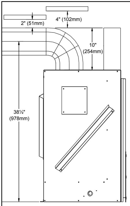
**Figure 23. Hard Vent Pipe Clearances.**
