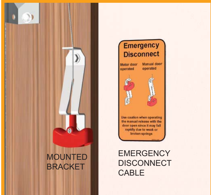
MANUAL DOOR OPERATED POSITION
