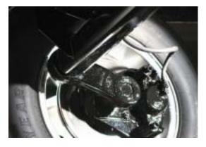
Your MasterCraft trailer brakes are designed to operate automatically when the tow vehicle's brakes are applied. These are known as surge brakes. When the tow vehicle slows down or stops, the forward momentum (*surge*) of the trailer against the hitch ball applies pressure to a master cylinder in the trailer coupler. This pressure acti-
