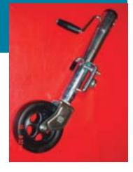
Like any mechanical assembly, a jack requires maintenance to function properly over a long period of time. The drive gear and the rack-and-pinion should be greased. The caster and wheel bearing should be oiled frequently. Failure to swing up the jack before towing may result in damage to your trailer.
