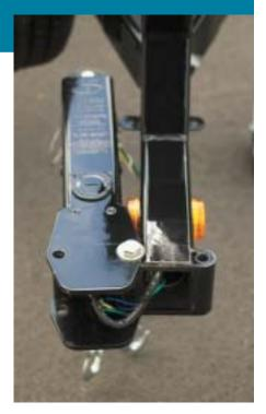
should not be more than 300 pounds, but not less than 150. (Some auto manufacturers say that tongue weight should not exceed 200 pounds when using a weight-carrying, bumper-mounted hitch with full-sized cars.)
