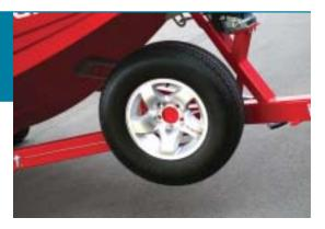
tire's sidewalls. Always check the air pressure when the tires are cold. Tires heat up and the air pressure increases after traveling short distances. Inflate tires to the proper air pressure as noted on the sidewall of the tires.
