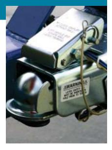
detached from the tow vehicle while traveling, which may cause serious injury or death or property damage. The coupling should not be allowed to lay on the ground where dirt or sand can enter the socket. This can cause excessive wear when the trailer is towed again, or it can cause the locking mechanism to jam.
