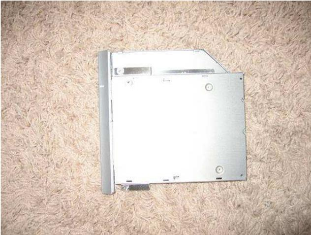
6. Remove the 3 black screws underneath the DVD drive. Note the size of the screws.
