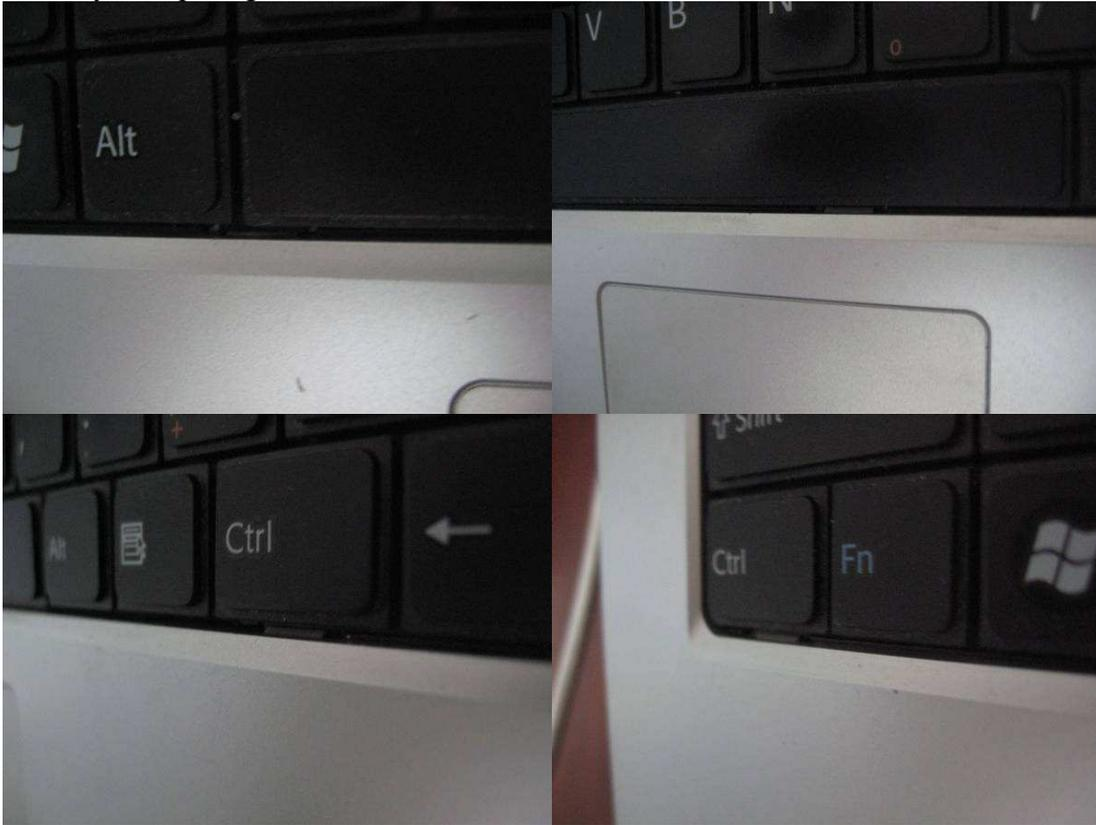
9. When you press in plastic tabs, carefully lift up on front black edge of keyboard.
