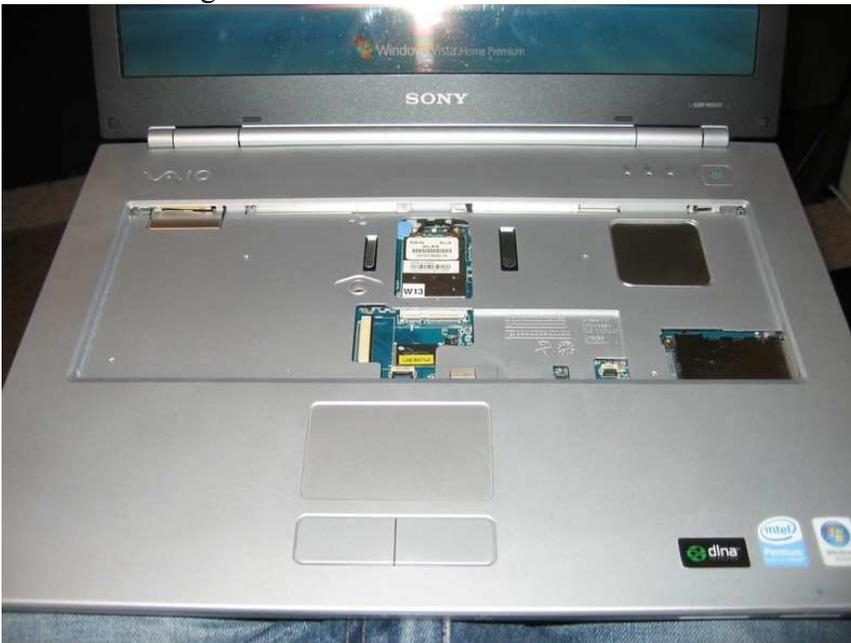
13. Remove the mouse touchpad ribbon cable by lifting up on the black part of the black and white connector. Pull the blue tab on the ribbon cable.
