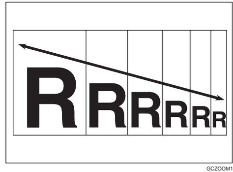
**Size Magnification (inch)—Fitting the original to a copy of a different size**
