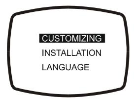
"P+", "P-" are used to move up & down in the main menu as the other pages. "+" or "-" is used to enter the sub-menus in the main menu. Exiting from this menu is only made by the "TV", "Store" and "Standby" buttons.
