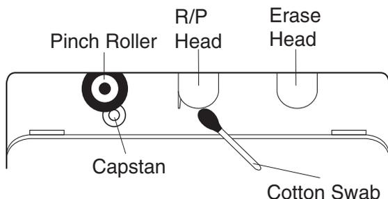
**NOTE:** Never use metal objects on or near the tape heads. Do not allow any cleaning material to fall into the tape assembly.
