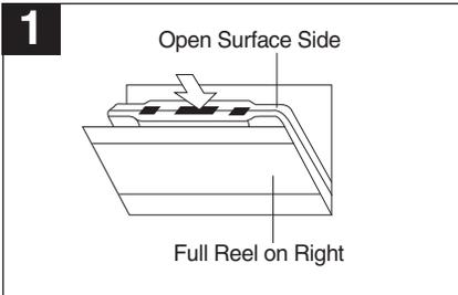
1 Open the Cassette Door and insert a good quality blank cassette tape into the slots on the door, with the open end facing up and the full reel on the right side. Close the Cassette Door.
