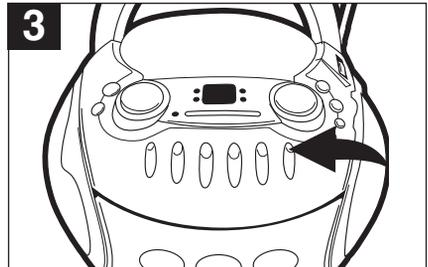
3 When you are ready to begin recording, press the RECORD (●) button. The PLAY (◀) button will also engage. The tape will begin moving and all of the material from your selected source will be recorded on the tape.
