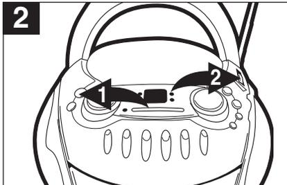
2 Press the POWER button ❶ to the in position and slide the Function switch ❷ to select the function you wish to record, either CD, AM or FM, and operate that function according to its own instructions.
