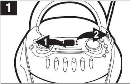
Press the POWER button ❶ to the in position and slide the Function switch ❷ to the CD position. Insert a CD as described in the TO INSERT A CD section on page 6.
