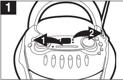
Press the **POWER** button ❶ to the in position and slide the **Function** switch ❷ to select AM or FM; the **POWER** indicator will light.
