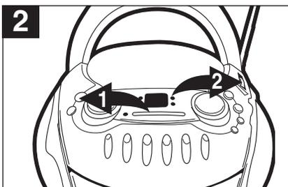
Press the **POWER** button ❶ to the in position and slide the **Function** switch ❷ to select CD; the **POWER** indicator will light.
