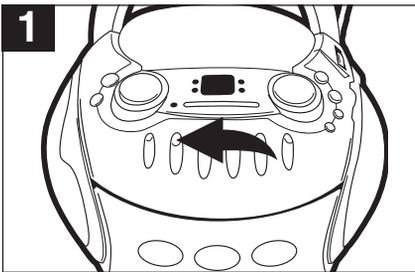
Press the STOP/EJECT (■) button to open the cassette compartment.
