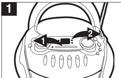
Press the POWER button ❶ to the in position and slide the Function switch ❷ to the CD position; the POWER indicator will light. Insert a CD as described in the TO INSERT A CD section on page 6.
