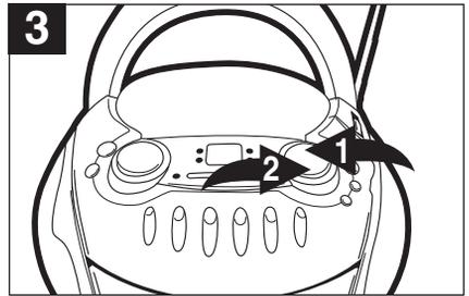
Press the PLAY/PAUSE button ❶ to begin playback and the unit will play the entire disc over and over until the STOP (■) button ❷ is pressed.
