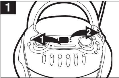
Press the POWER button ❶ to the in position and slide the Function switch ❷ to the CD position and insert a CD as described in the TO INSERT A CD section on page 6.
