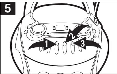
To advance or rewind the tape rapidly, press either the F.FWD (◀◀) ❶ or REWIND (▶▶) ❷ button. When you reach the desired point, press the PLAY (◀) button ❸ to resume normal playback.
