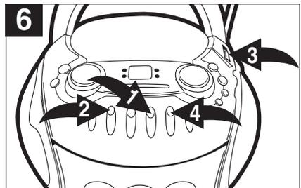
6 If you wish to listen to your recording immediately, press the cassette REWIND (▶▶) button ❶ until the tape rewinds to the beginning, then press the STOP/EJECT (■) button ❷. Slide the Function switch ❸ to the TAPE/POWER OFF position, then press the PLAY (◀) button ❹ to begin playback.
