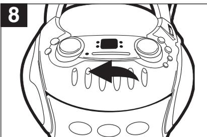
When the tape reaches the end, the auto-stop mechanism activates, the PLAY (◀) button is released and the tape motor shuts off. Press the STOP/EJECT (■) button to open the cassette compartment and remove the cassette.
