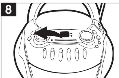
To turn the radio off, press the POWER button again; the POWER indicator will go off.
