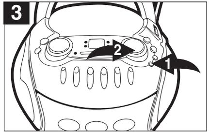
Press the REPEAT button ❶ once, the REPEAT indicator will blink and the unit will play the selected track over and over until the STOP (■) button ❷ is pressed.
