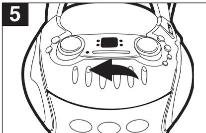
5 When you are finished recording, press the STOP/EJECT (■) button to stop the tape.
