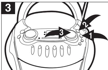
To start from a specific track, locate the track using the SKIP/Search (⏮) ❶ or (⏭) ❷ button and press the PLAY/PAUSE (▶||) button ❸.
