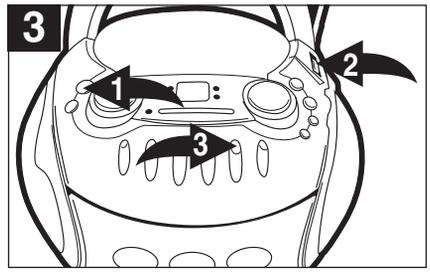
Press the POWER button ❶ to the in position and slide the Function switch ❷ to the TAPE position, then press the PLAY (◀) button ❸ to begin playback.
