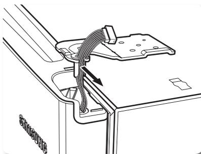
5. Separate Hinge from electric wire and ground wire as shown above.
