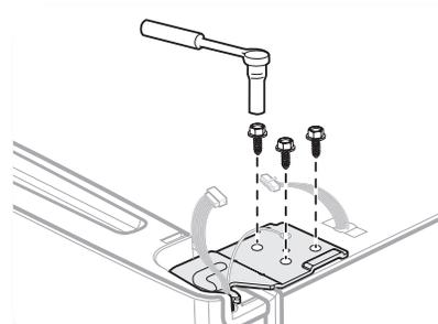
3. With the 7/16 inch wrench, remove the three bolts that hold the hinge on the top of the refrigerator.
