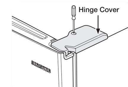
1. After removing the screw, remove the upper Hinge Cover.
