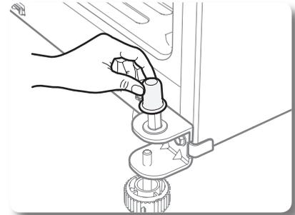
5. Remove the Cap on the Bottom Hinge.
