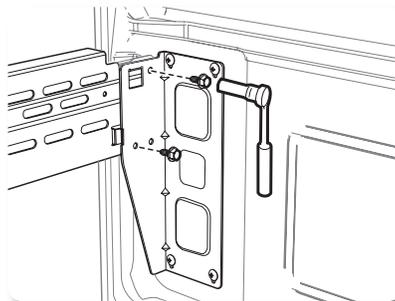
4. With the 7/16inch wrench, remove two bolts connecting the rail with the door.
