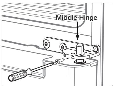
2. After removing one screw and two bolts, remove the Middle Hinge. (Unscrew the screws with the screwdriver(+) and hex bolts with the 3/16inch hex wrench.)
