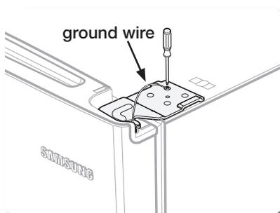
4. Remove the screw that holds the ground wire.
