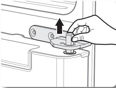
3. Remove the Middle Hinge connected to the Freezer.
