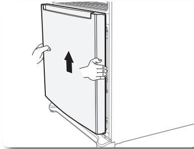
4. Remove the Freezer door by lifting it upward.
