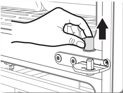
1. Separate the Cap on the Middle Hinge.
