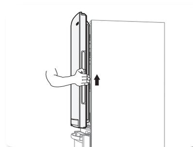
6. Remove the fridge door by lifting it upward.
