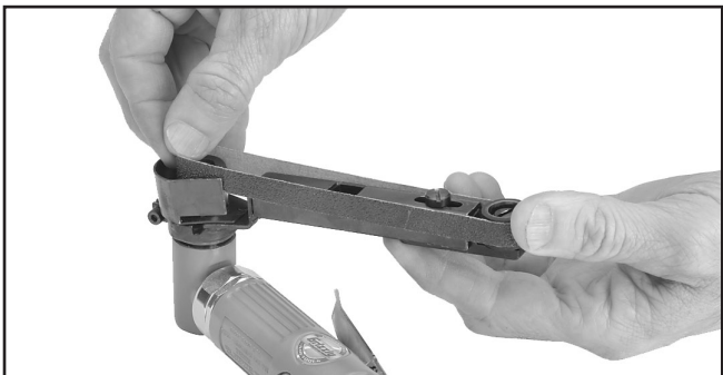
Figure 5. Installing sanding belt.
