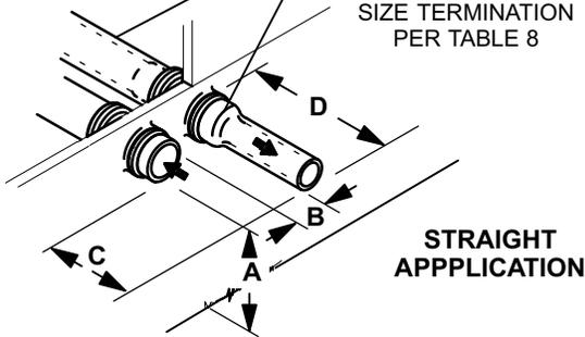
1/2" (13mm) ARMAFLEX INSULATION IN UNCONDITIONED SPACE
