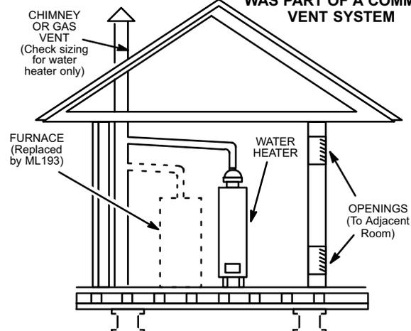
If an ML193DF furnace replaces a furnace which was commonly vented with another gas appliance, the size of the existing vent pipe for that gas appliance must be checked. Without the heat of the original furnace flue products, the existing vent pipe is probably oversized for the single water heater or other appliance. The vent should be checked for proper draw with the remaining appliance.
