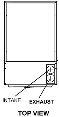
\* When transitioning up in pipe size, use the shortest length of 2" PVC pipe possible.
