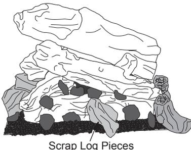
**Figure 31 - Installing Scrap Log Pieces**
