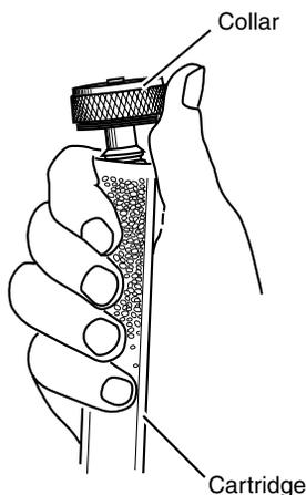
The desiccant is contained in a cartridge located on the left side of the 2150EX. To remove the cartridge, unscrew the collar and slide the cartridge out of the 2150EX. The opaque tube reveals the silica gel desiccant inside.
