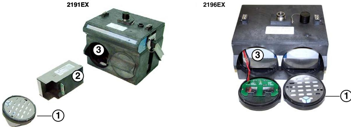
Figure 1-4 2191EX and 2196EX Battery Components
