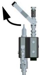
4. Open the solvent inlet valve (C). For the quickset manifold, close the A side flush valve (T).
