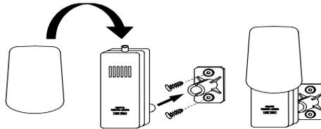
7. Screw mounting bracket onto the mounting surface. The screws should be flush with the bracket.
