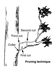
Make the first cut 6 inches (15 cm) from the tree trunk on the bottom of the limb. Use top of guide bar to make this cut. Cut 1/3 through the diameter of the limb.
