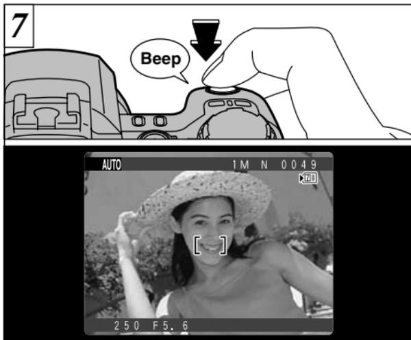
If you press the shutter button down halfway and then press the shutter button down fully without releasing it, the camera beeps once and takes the picture. The “
