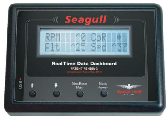
**Variometer Function:** Your Dashboard contains a sophisticated Variometer, employing electronic Total Energy Compensation, based on changes in Airspeed. Basic variometers do not support total energy, which means that "stick thermals" are reported by the variometer if you descend or ascend due to elevator movement. Standard total energy variometers reduce the effects of moving the
