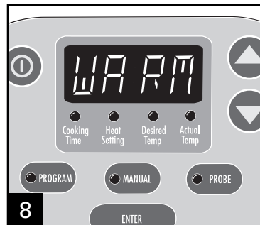
8 At the end of the cook time, the slow cooker will automatically switch to the Keep Warm setting. NOTE: Unit will turn off and display OFF after a total of 14 hours.
