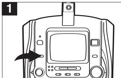
During playback, press the INTRO button; the INTRO indicator will light and the unit will then play the first 10 seconds of each track and then stop.
