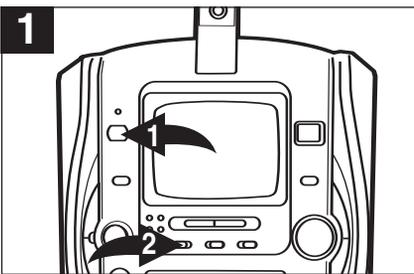
Press the POWER button ❶ to turn the unit on. Slide the FUNCTION switch ❷ to the CDG position.
