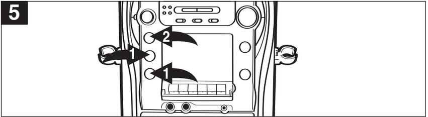
5 Adjust the MIC VOLUME controls 1 as desired. Increasing this control will increase the volume of the microphone. Adjust the ECHO control 2 to add an echo effect to your voice. The ECHO control 2 is variable so add as much or as little reverb as desired. Sing or talk into the microphone and you will hear both the CD+G and the microphone.
