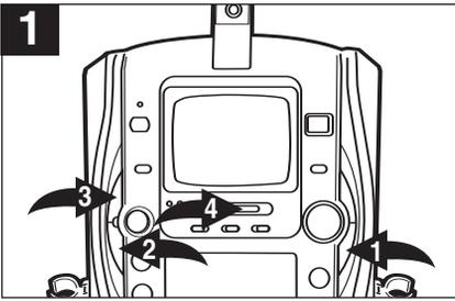
To repeat a single track, while in the Stop mode, press the REPEAT button ❶ once; the REPEAT indicator will blink. Press the SKIP/SEARCH ◀▶ ❷ or ▶▶ ❸ button to select the specific track that you wish to repeat. When the desired track number blinks in the display, within five seconds, press the PLAY/PAUSE (▶||) button ❹ to begin playback. The specific track you selected will be repeated continuously.
