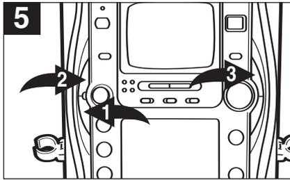
Press either the SKIP/SEARCH **1** or **2** button to select the next track you wish to program. When the desired track number appears in the display, press the PROGRAM button **3** again.
