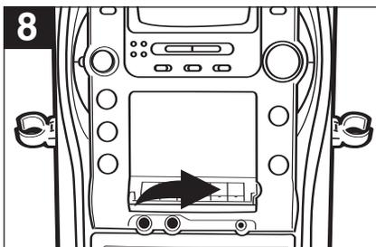
When the tape reaches the end, the auto-stop mechanism activates, the **PLAY** (▶) button is released and the tape motor shuts off. Press the **STOP/EJECT** (■▲) button to open the cassette door and remove the tape.
