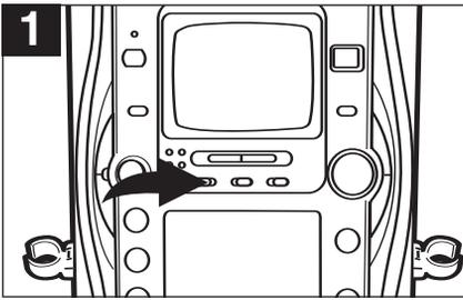
Slide the **FUNCTION** switch to the **TAPE** position. Open the cassette button compartment to expose the cassette buttons.
