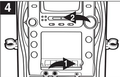
4 Press the PAUSE (||) button ❶ to release pause and then press the CD PLAY/PAUSE (▶||) button ❷ to start CD/CD+G playback.
