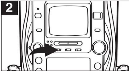
2 Slide the FUNCTION switch to the CDG position. Insert the microphone into the appropriate jack.
