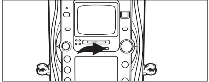
Slide the MONITOR switch to select what image will appear on the built-in monitor:
