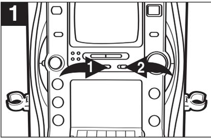
Slide the VIDEO OUT switch ❶ to the CAMERA position to see the camera's image on the external TV. Slide the MONITOR switch ❷ to the CAMERA position to see the camera's image on the monitor.
