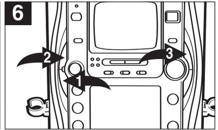
Repeat step 5 until you have programmed the desired track numbers into the CD Program Memory. When the memory is full, "- -" will blink in the display.
