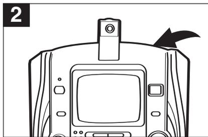
Lift up the LIFT TO OPEN area to open the CD compartment door. Place a CD in the compartment, with the printed label side facing up and close the CD compartment door.
