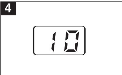
4 The CD player will read the table of contents on the disc and the total number of tracks on the disc will appear in the display.
