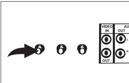
If the picture moves up and down or rolls, rotate to adjust the vertical hold.
