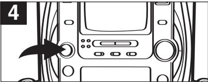
4 Rotate the AUTO VOICE control clockwise to suppress the vocal tracks on the CD being played when singing into the microphone. Rotate the AUTO VOICE control counterclockwise to have the vocal tracks on the CD play at normal volume.
