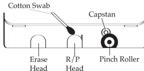
**NOTE:** Never use metal objects on or near the tape heads. Do not allow any cleaning material to fall into the tape assembly.
