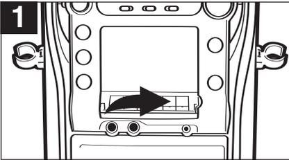
1 Press the STOP/EJECT (■▲) button to open the cassette door and insert a cassette with the open end facing down. Close cassette door.
