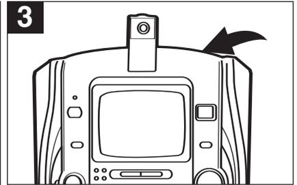
3 Lift up the LIFT TO OPEN area to open the CD compartment door. Place a CD in the compartment, with the printed label side facing up and close the CD compartment door.
