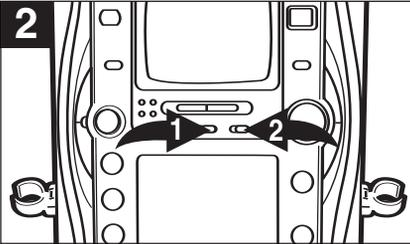
2 Slide the VIDEO OUT switch 1 to the CDG position to see the CD+G lyrics on the external TV. Slide the MONITOR switch 2 to the CDG position to see the CD+G lyrics on the monitor.
