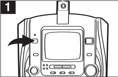
1 Press the POWER button to turn the unit on; the POWER indicator will light.
