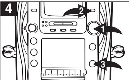
Adjust the **MASTER VOLUME** control ❶, **MEGA BASS** button ❷ and **PITCH** control ❸ as desired.
