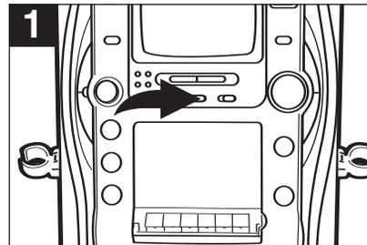
To output this unit's video/audio onto the unit connected to the A/V OUT jacks. Slide to the CDG position when viewing/listening to a CDG or CDs, slide to the AUX position when listening to the unit connected to the A/V IN jacks on the rear of the unit or slide to the CAMERA position to view the camera's image.
