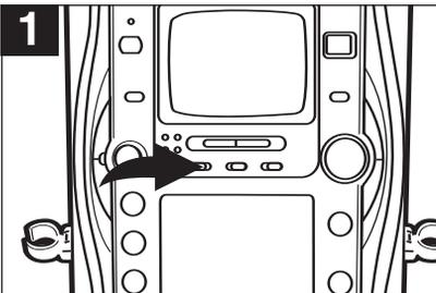
Slide to the CDG position when using CDG or CDs, slide to the TAPE position when playing tapes or slide to the AUX position when listening to the unit connected to the A/V IN jacks on the rear of the unit.
