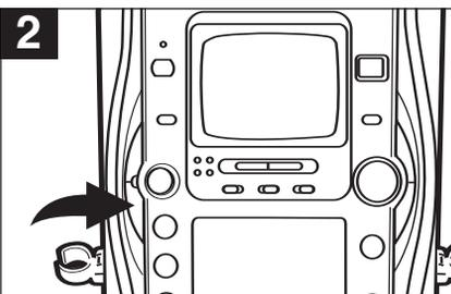
During playback, press the SKIP/SEARCH (◀◀) button once to move the player back to the beginning of the current track. Press the SKIP/SEARCH (◀◀) button repeatedly to move the player back to lower-numbered tracks.
