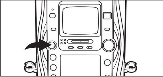
When the AVC feature is activated, the vocals on a multiplex recording are muted as soon as the singer begins singing into the microphone. When the singer stops singing, the vocals are automatically un-muted. Adjust AVC control for the best balance between playback and microphone levels.
