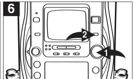
6 Adjust the MASTER VOLUME control ① and MEGA BASS button ② as desired. Playback will continue until all of the tracks on the disc have been played.
