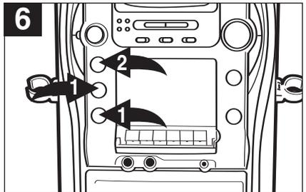
6 Adjust the MIC1/MIC2 VOLUME controls ❶ as desired. Increasing this control will increase the volume of the respective microphone. Adjust the ECHO control ❷ to add an echo effect to your voice. The ECHO control ❷ is variable so add as much or as little reverb as desired.
