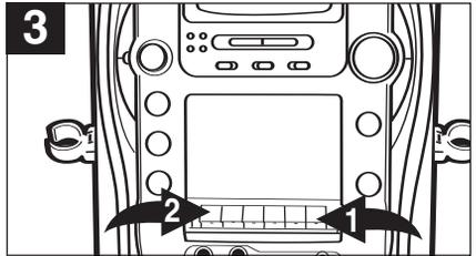
3 Press the PAUSE (||) button ❶, then press the RECORD (●) button ❷ (the PLAY (▶) button will be automatically depressed).
