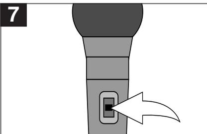
7 Turn the microphone on using the Microphone ON/OFF switch. Sing or talk into the microphone(s) and both the CD/CD+G and the microphone(s) will be recorded onto the cassette.
