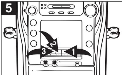
To advance or rewind the tape rapidly, press either the **FFWD** (▶▶) ❶ or **REWIND** (◀◀) ❷ button. When you reach the desired point, press the **PLAY** (▶) button ❸ to resume normal playback.
