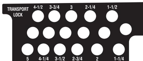
The deck height index consists of several holes located on the front/right of the foot platform. Each hole corresponds to a 1/4" change in the deck height position ranging from 1" at the lowest notch to 5" at the highest notch.
