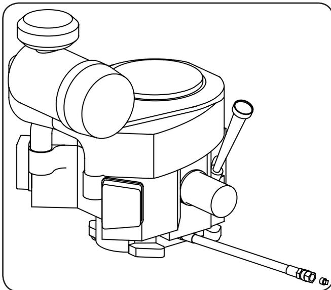
5. After draining the oil, wipe any residual oil from the oil drain hose. Thread the square head plug into the drain hose fitting and fully tighten the plug.
