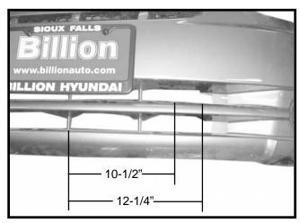
16. Cut outside grill bar on facia by measuring from the center bar as shown in picture. NOTE: Some trimming maybe needed for base plate to pass through.
