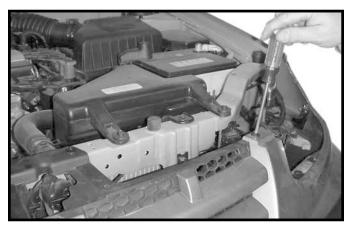
**2.** Open hood and remove four plastic push fasteners from top of facia.
