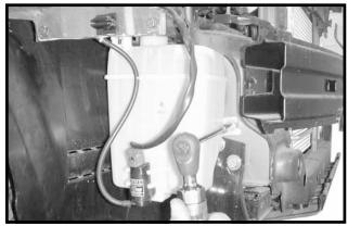
**11.** Remove three bolts from windshield washer tank, unplug wiring and hose, and set tank aside or tie off.
