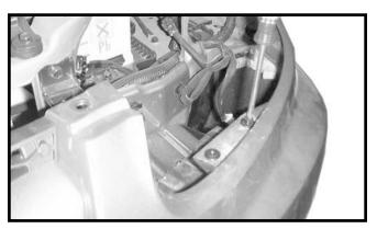
**5.** Remove two plastic push fasteners from underneath headlight (top of facia) on each side.
