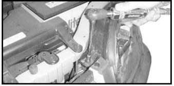
**1.** Remove two bolts that hold headlights and unplug headlights and set aside.
