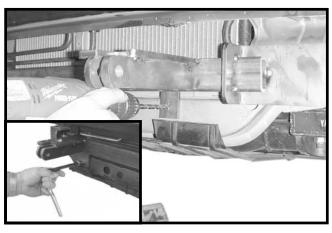
**14.** Drill two 5/16" holes, one through each center base plate tabs. With blue **LOCTITE** on each 3/8" self-tapping bolts, install through drilled holes.
