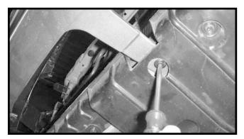
Remove two plastic push fasteners from bottom of facia.
