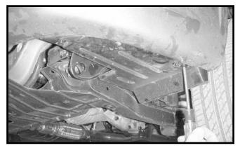
**8.** Remove two plastic push fasteners from each side underneath facia to inner wheel well extension.
