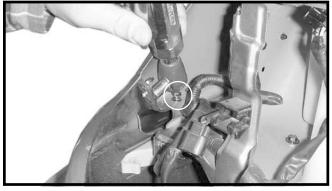
3. Remove one nut and one bolt from fasia to fender on each side.
