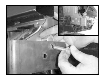
13. Slide base plate on passenger's side first, then pivot over driver's side. Use three 12mm-1.25 x 35mm bolts and 12 mm lock washers on passenger's side using blue LOCTITE. on all bolts. On driver's side, use three 12mm-1.25 x 70mm bolts, 12mm lock washers, and put three spacer bushings behind baseplate up against frame. Push base plate back against vehicle so center tabs of base plate are tight against vehicle. Tighten the six 12mm bolts.
