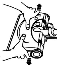
4. Lift rear latches up and tilt cover forward from back until front snaps free.
