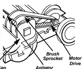
3. Place agitator assembly back into the Power Brush.
