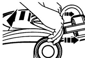
5. Depress tabs on rear of agitator cover and rotate forward to release from the base of the Power Brush.
