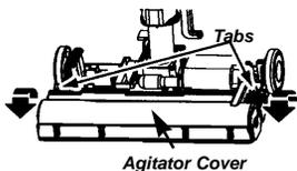
6. Lift agitator assembly out and remove worn belt.
