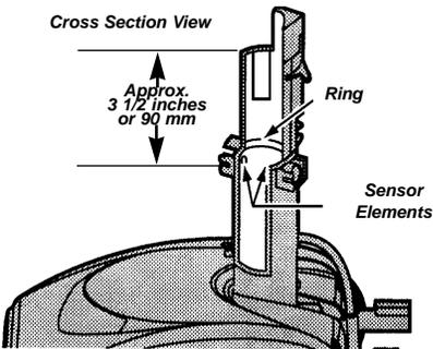
2. As indicated by the illustration, the two dirt sensor elements are located on the sides of the swivel, approximately 3 1/2 inches/90 mm down, (note the arrows). Each element should be cleaned periodically. To reach the sensor elements, use a small brush such as a bottle brush. Brush each sensor element several times to remove dust and dirt.
