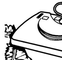
**To correct problem:** Turn off vacuum, remove obstruction, then press reset button.
