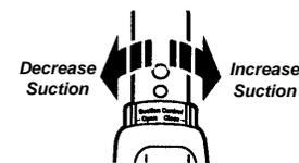
Opening the control decreases suction for draperies and lightweight rugs, while closing the control increases suction for upholsteries and carpets.
