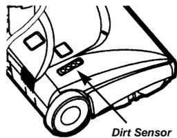
The lights give you an indication of the amount of dirt particles that are passing thru the sensor on its way to the dust bag.
