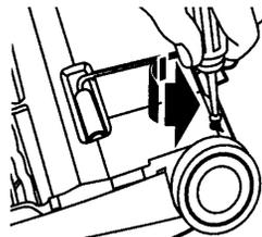
3. Turn the Power Brush right side up. Press handle release pedal and lower the swivel. To remove cover, grasp the sides and pull out to release the outside of the cover.
