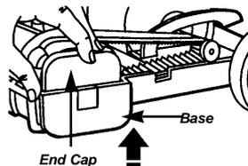
7. Slide end caps off to check and clean end cap areas. See page 12 for picture of complete agitator assembly.
