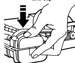
4. Replace agitator cover by lining up the front tabs and slots and rotating downward until the latches snap into place.
