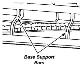
When brushes are worn to the level of the base support bars, replace the agitator assembly.
