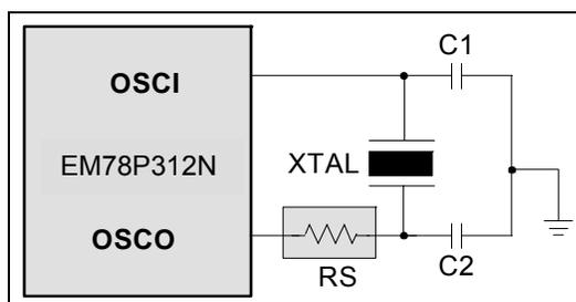
Fig. 5-30 Crystal/Resonator Circuit
