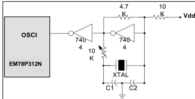
Fig. 5-32 Crystal/Resonator-Parallel Mode Circuit
