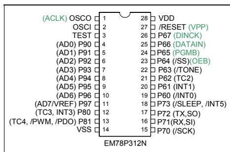
Fig. 3- Pin Assignment
