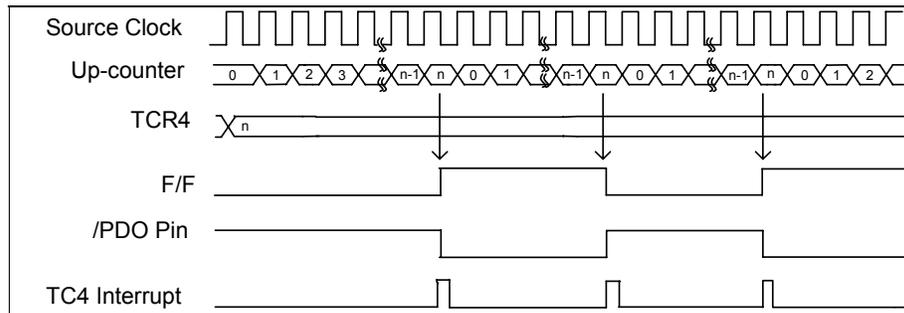
Fig. 5-25 Timing Chart for PDO Mode
