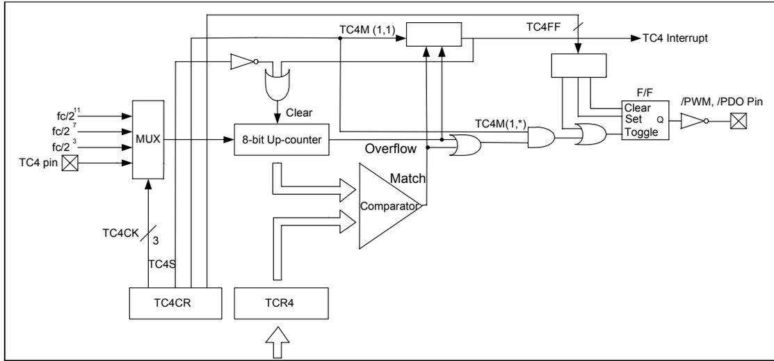
Fig. 5-24 Timer/Counter 4 Configuration
