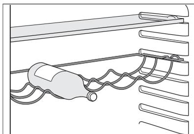
This bottle holder shelf can be tilted in order to store previously opened bottles. To obtain this result, pull the shelf up so it can rotate upwards and be placed on the next higher level.
