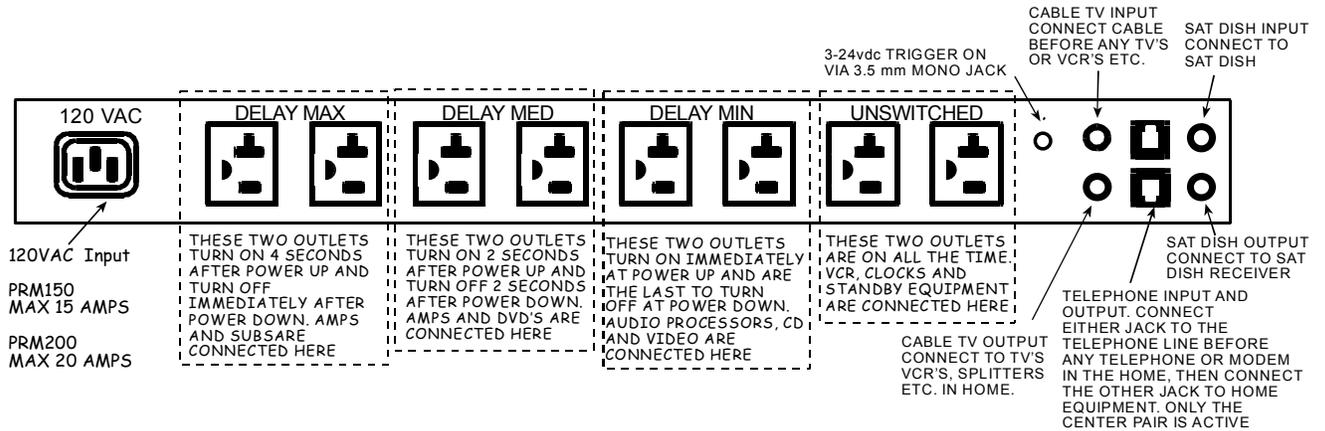
The PRM150 requires a dedicated properly grounded 15-amp circuit to operate at capacity. We suggest that a dedicated 15-amp breaker be installed at the breaker box for use with the PRM150.
