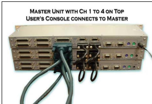
FIGURE 3 Stacking of MC4-H2 Units
