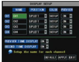
From the Main Menu, select CAMERA. Here you can setup the name display (up to 8 characters) and position of each channel (camera). Select COLOR SETUP to adjust the image brightness, saturation, contrast and hue settings of each channel (camera). You can also choose whether each channel can be previewed in LIVE MODE and/or RECORDING MODE.
