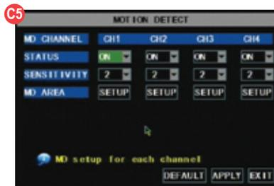
The Motion detection Menu (C5) has three sections, including Channel Status, Sensitivity and Motion area.
