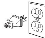
**CAUTION:** To prevent electric shock, match wide blade of plug to wide slot, fully insert.
