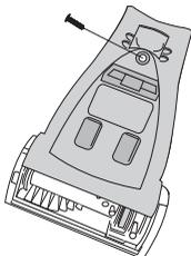
2) Rotate lower part of cover down over brush and lift off cover.
