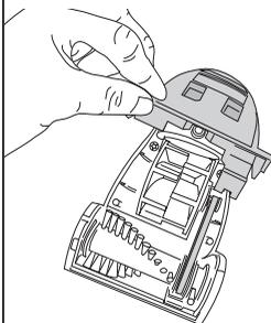
3) Clear blockage from brush roll area. Use scissors to clip threads or hair.
