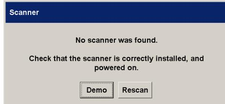
1. Check that the scanner power is ON.
