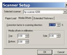
Positive settings mean that the distance between scan lines will be increased, and negative settings mean that the distance between scan lines will be decreased.
