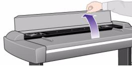
2. Press down on the platen as you pull first one slider and then the other (left and right) towards the scanner's center until the media thickness adjustment sliders found at each side are the same setting.
