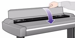
To return the insertion slot height to its Normal position:
