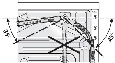
2. Connect the hose with a straight connection to a water tap with a screw thread R 3/4 (inches).
