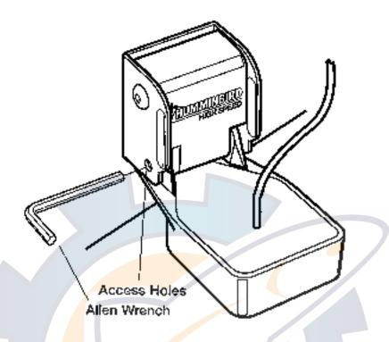
Note: On some hulls, it may be necessary to angle the transducer so that the back end is 1/4" lower than the front.
