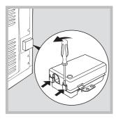
supply cable by loosening the cable clamp screw and the three wire contact screws L-N-\(\frac{1}{2}\). Connect the wires to the corresponding terminals: the Blue wire to the terminal marked (N), the Brown wire to the terminal marked (L) and the Yellow/Green
