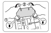
To temporarily place the handset down during a conversation, hook it over the top edge of the phone as shown.
