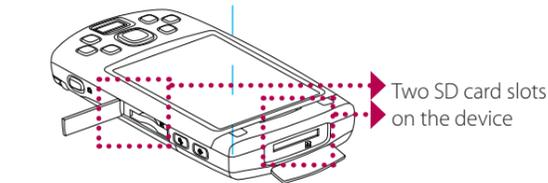
Peel open the rubber that covers the storage card slot and insert the SD card into the slot with its gold contacts facing down.
