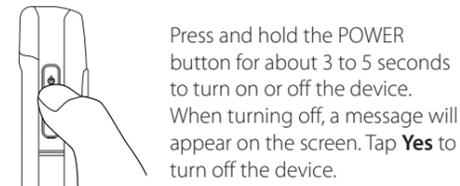
Press and hold the POWER button for about 3 to 5 seconds to turn on or off the device. When turning off, a message will appear on the screen. Tap **Yes** to turn off the device.
