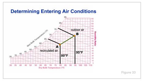
If outdoor air **B** is mixed with recirculated air **A**, the conditions of the resulting mixture are found somewhere on a straight line connecting the two points.
