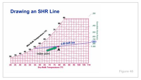
Assume that room design conditions (**A**) are 78°F DB and 65°F WB, and that the sensible heat ratio is calculated as 0.80. That is, sensible heat gain represents 80% of the total (sensible plus latent) heat gain.
