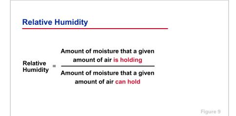
The fourth property, **relative humidity**, is a comparison of the amount of moisture that a given amount of air *is* holding, to the amount of moisture that the same amount of air *can* hold, at the same dry-bulb temperature.
