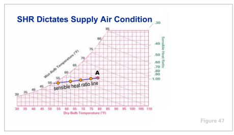
Supply air with any combination of dry-bulb and wet-bulb temperatures that falls on this line will be able to absorb the room's sensible and latent heat in the correct proportions needed to maintain the desired room conditions ( $\mathbf{A} = 78^{\circ}\text{F DB}$ , 65°F WB).
