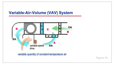
The final method of part-load control we will analyze is to vary the supply airflow to the room.
