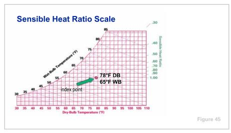
A scale around the right and top edges of the chart gives the SHR values. Also, there is an **index point** in the middle of the chart at the 78°F DB and 65°F WB condition.
