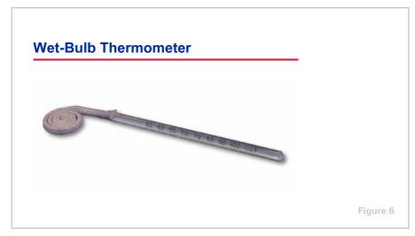
**Wet-bulb temperatures** are read from a thermometer whose bulb is covered by a wet wick. The difference between the wet-bulb temperature and the drybulb temperature is caused by the cooling effect produced by the evaporation of moisture from the wick. This evaporation effect reduces the temperature of the bulb and, therefore, the thermometer reading.
