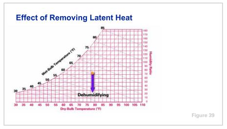
Conversely, if only latent heat is removed, the line moves vertically downward along a constant dry-bulb temperature line. This results in a lower moisture content or humidity ratio.
