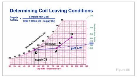
After determining the entering air conditions for the coil and the slope of the SHR line, the **coil curves** were used to find the required supply air conditions. This point (**D**) was established by the intersection of the coil curve and the SHR line.
