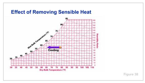
If only sensible heat is removed from the air, the line representing this change moves from the original condition horizontally to the left. This results in a lower dry-bulb temperature, while the moisture content (the humidity ratio) remains constant.
