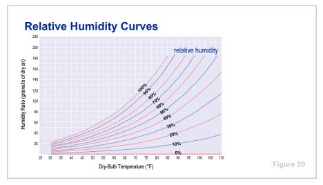
Additional curves can be added to the chart to represent relative humidity conditions that are less than 100%. The curves shown are at 10% intervals and represent humidity conditions ranging from completely saturated air to completely dry air. When air is completely dry, its relative humidity cannot change with temperature. The 0% condition is therefore represented by the horizontal axis of the chart.
