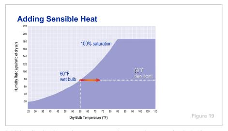
Additionally, the dew-point temperature does not change as the dry-bulb temperature changes, provided that the moisture content of the air remains the same. Merely heating the air does not change its moisture content. Therefore, as the air is heated, its condition will move horizontally along a constant humidity-ratio line.
