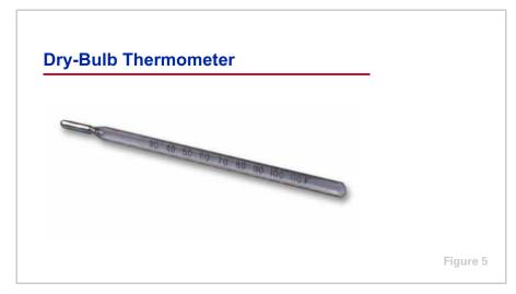
**Dry-bulb temperatures** are read from an ordinary thermometer that has a dry bulb.
