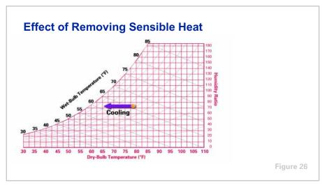
Conversely, if sensible heat is removed from air, the air condition moves horizontally to the left. As long as the moisture content of the air remains unchanged, the humidity ratio remains the same. Therefore, this movement follows the horizontal humidity-ratio lines.
