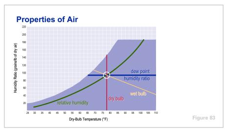
The lines of the psychrometric chart represent five physical properties of air: **dry bulb, wet bulb, dew point, humidity ratio,** and **relative humidity**. If any two of these properties are known, the remaining properties can be determined from the chart.
