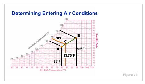
Returning to the psychrometric chart, point **C**, at which the 83.75°F dry-bulb temperature falls on the line from **A** to **B**, represents the conditions of the air mixture: 83.75°F DB and approximately 70°F WB.
