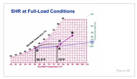
In the previous example, the sensible heat ratio was based on **full load or design load conditions**. It must be understood that the sensible portion of total heat gain is particularly subject to change throughout the day, causing the ratio of sensible to total heat gain to change.
