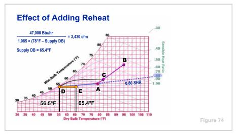
Using the part-load conditions from the previous example, the room's sensible heat gain is reduced from 80,000 Btu/hr to 47,000 Btu/hr while the latent heat gain remains the same.
