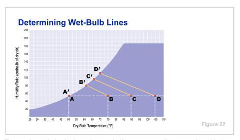
To complete this basic chart, the wet-bulb temperature lines must be added.
