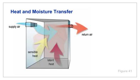
Imagine conditioned supply air as a sponge. As it enters a room, it absorbs heat and moisture. The amount of heat and moisture absorbed depends on the temperature and humidity of the supply air. This "sponge," the supply air, must be cool enough to pick up the room's excess sensible heat gain and dry enough to pick up the room's excess latent heat (i.e., moisture.)
