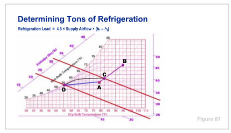
After the entering (**C**) and leaving (**D**) coil conditions were established, the **enthalpies** for each were read from the psychrometric chart. These enthalpy values and the previously calculated supply airflow were used to determine the **refrigeration load** in Btu/hr or tons.
