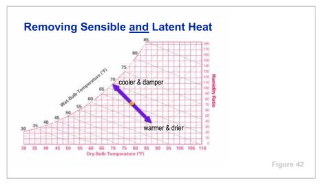
When the required amount of sensible and latent heat are not properly removed from the room, the desired room conditions cannot be maintained. For example, if too much sensible heat and not enough latent heat are removed, the room feels cold and damp. On the psychrometric chart, room conditions move up and to the left.
