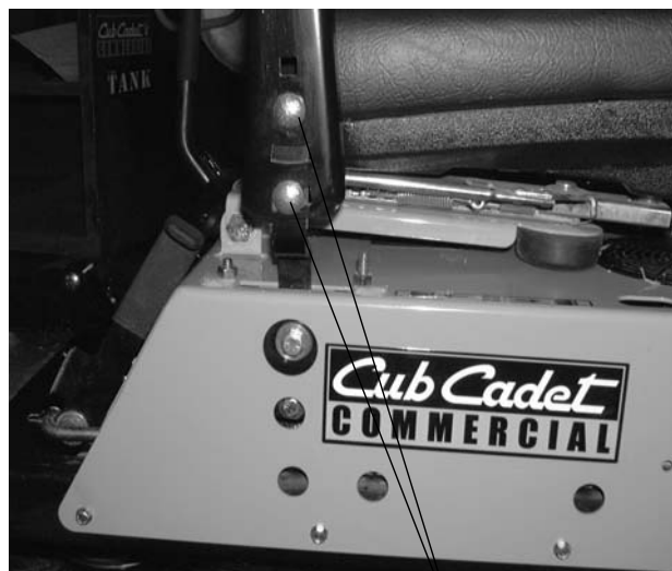
Figure. 10 Lap Bar Mounting Bolt and Nuts
